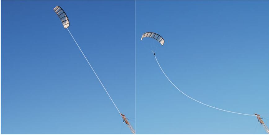
Fig. 7.9 Kite performing crosswind flight maneuvers with practically straight tether while reeling out (left) and non-maneuvering kite with strongly sagging tether while reeling in (right). Photographic footage with traced tether from 2 August 2012
