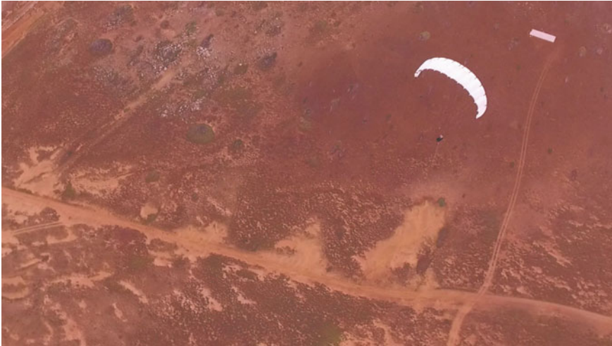
Fig. 7.1 Airborne wind energy system with 60\text{ m}^2 kite and suspended robotic control unit, operating on the Caribbean island Aruba in October 2021. Video still of the original drone footage with enhanced red tones (Schmehl 2022). Courtesy of Kitepower B.V.
