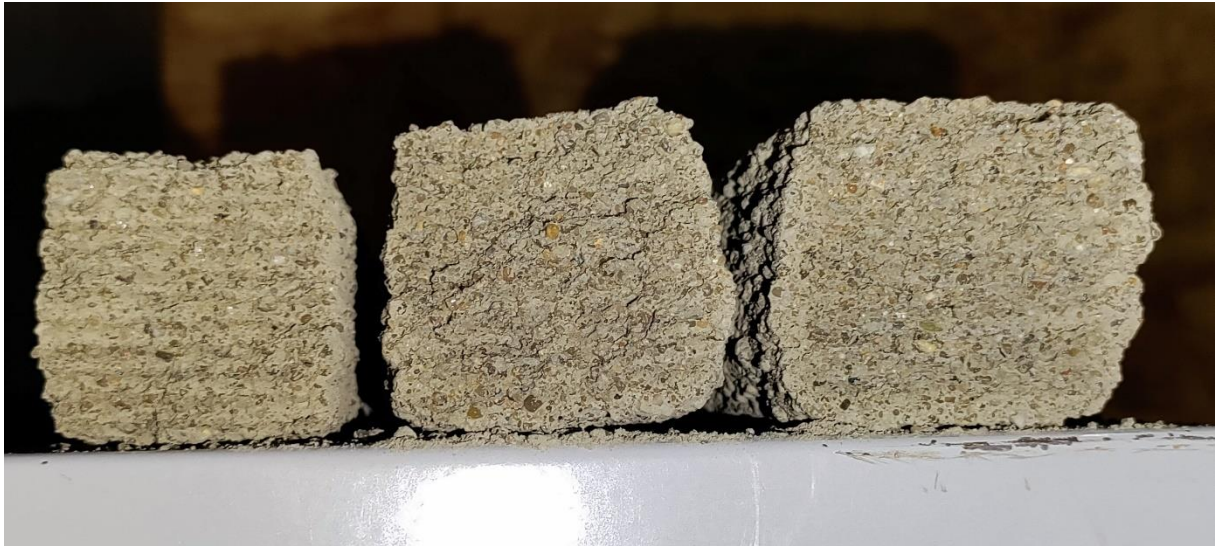
Figure 35: Cross sections of bending beams captured directly after failure. The beams are made using the 'linear' mix with water cement ratios of 0.2, 0.3 and 0.4 from left to right.
