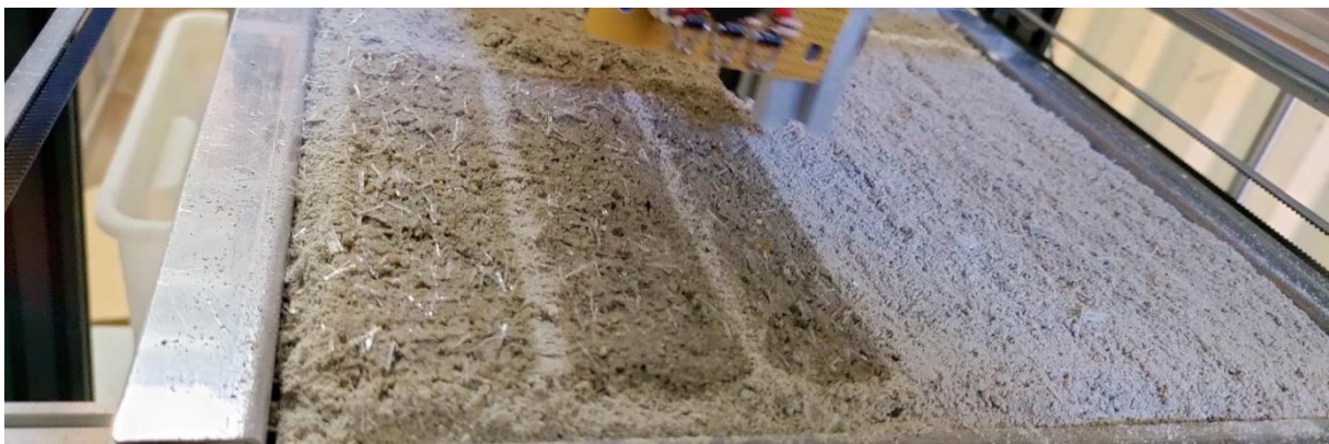
Figure 44: The uneven printing surface that occurs when printing with fibres
