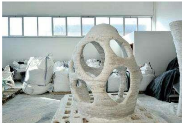
Figure 6: A 3D printed structure from D-shape made using a magnesium-based binder (Edwards, 2010)
