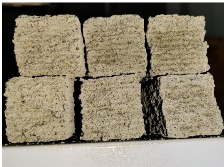
Figure 34: Photo of cross section of multiple bending test specimens taken directly after a bending test. Top row is 0.25% Tylose, bottom row contains 0.5% Tylose. The w/c ratio is increased from left to right
