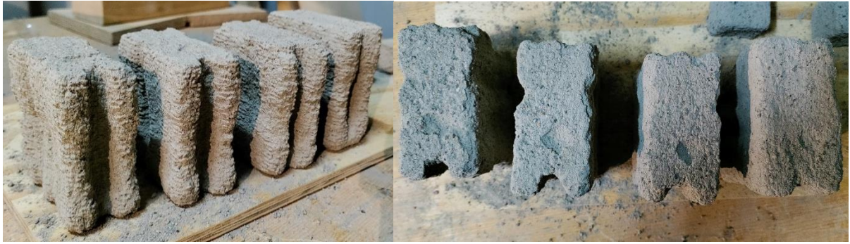
Figure 25: Test specimens with different w/c ratios to test dimensional accuracy. W/C ratio from left to right: 20,30,40,60 %
