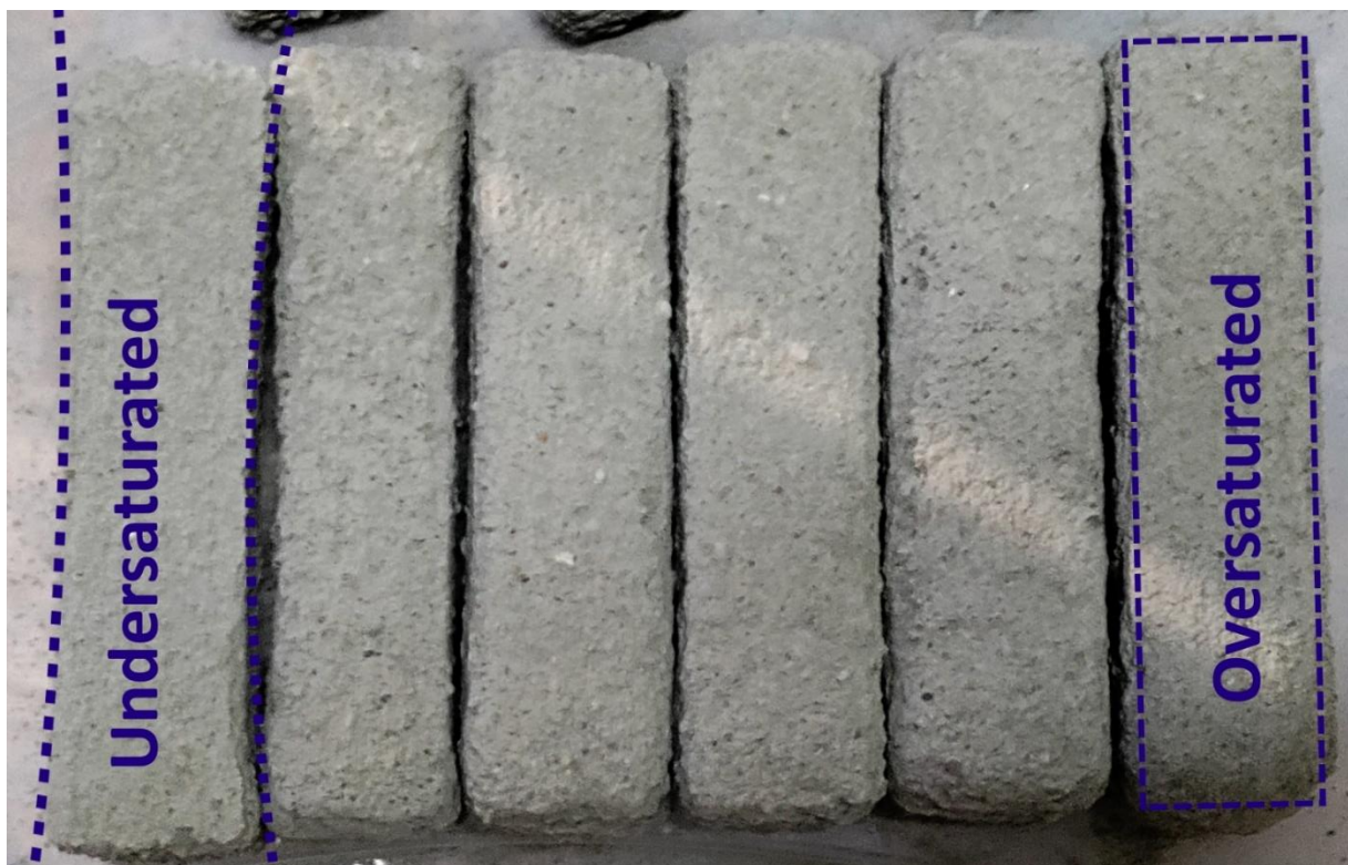
Figure 27: Undersaturation and oversaturation of the pore space in bending test specimens
