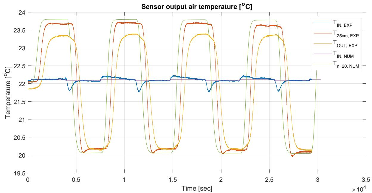
Figure 3.9: Comparison of experimental and numerical results for inlet and outlet air temperature.
