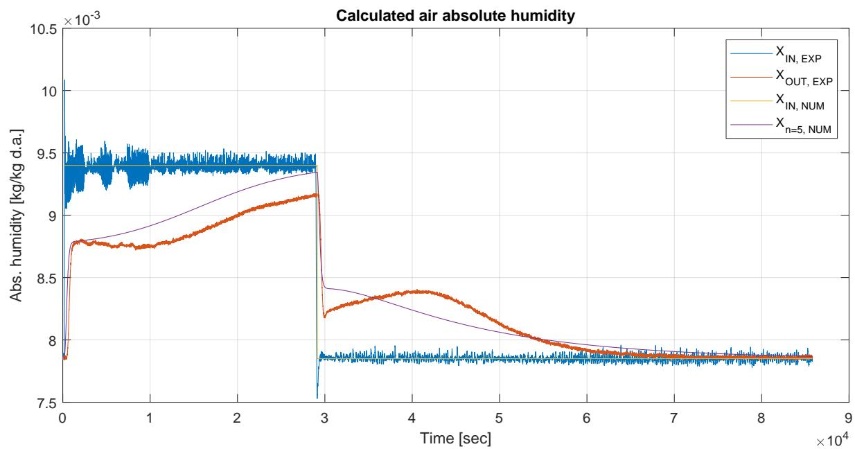
Figure 3.14: Comparison of experimental and numerical results for absolute air humidity at 13 cm and  $n = 5$ .
