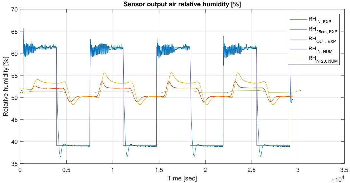
Figure 3.1: Comparison of experimental and numerical results for inlet and outlet relative air humidity.
