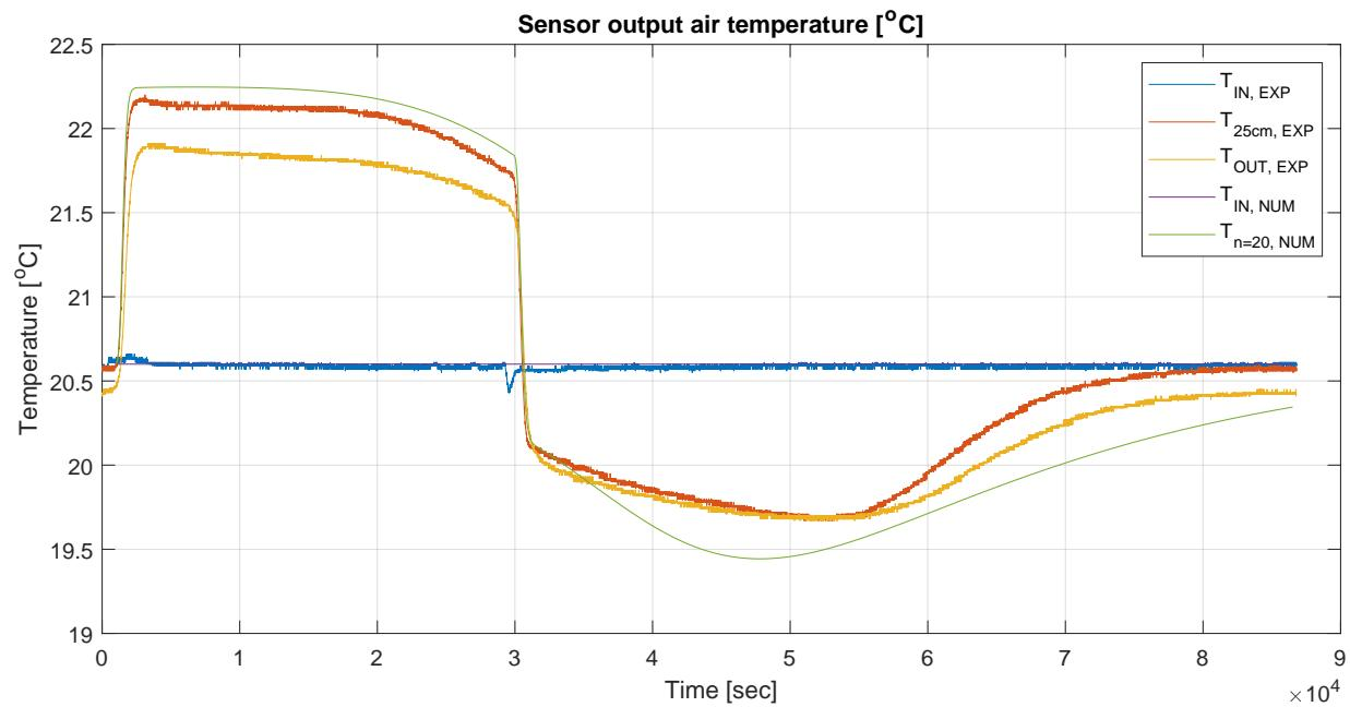
Figure 3.30: Comparison of experimental and numerical results for inlet and outlet air temperature.
