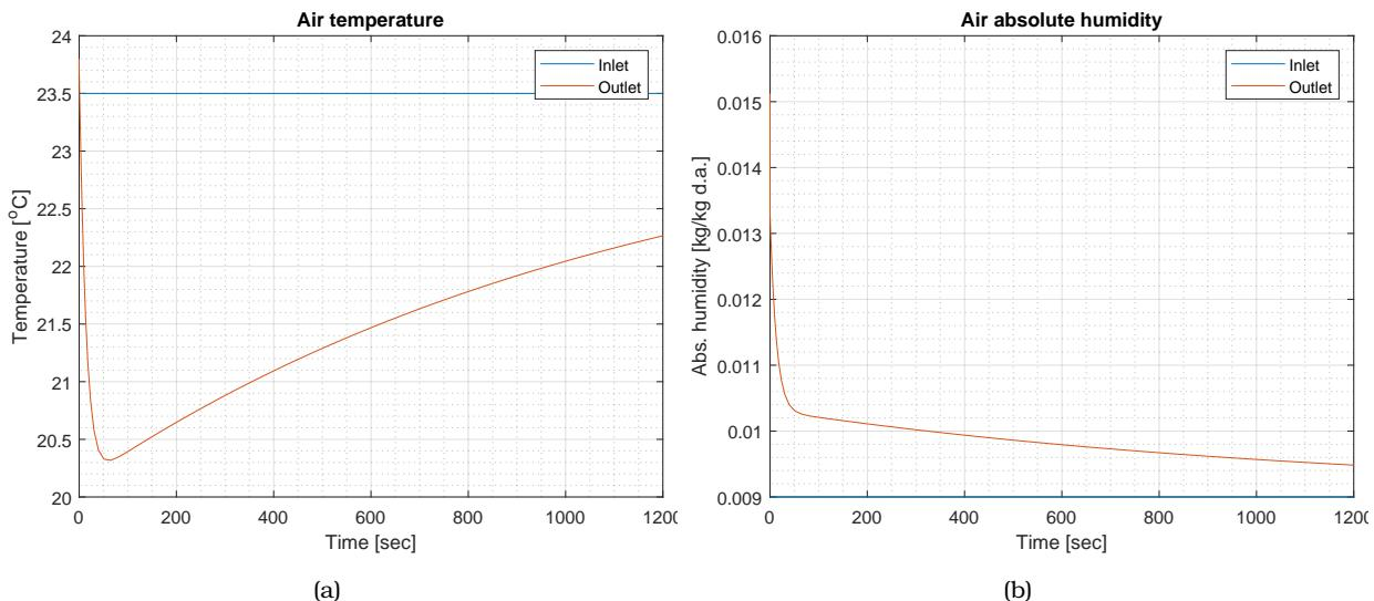
**Figure 2.11:** PGC model results for (a) air temperature and (b) absolute air humidity.
