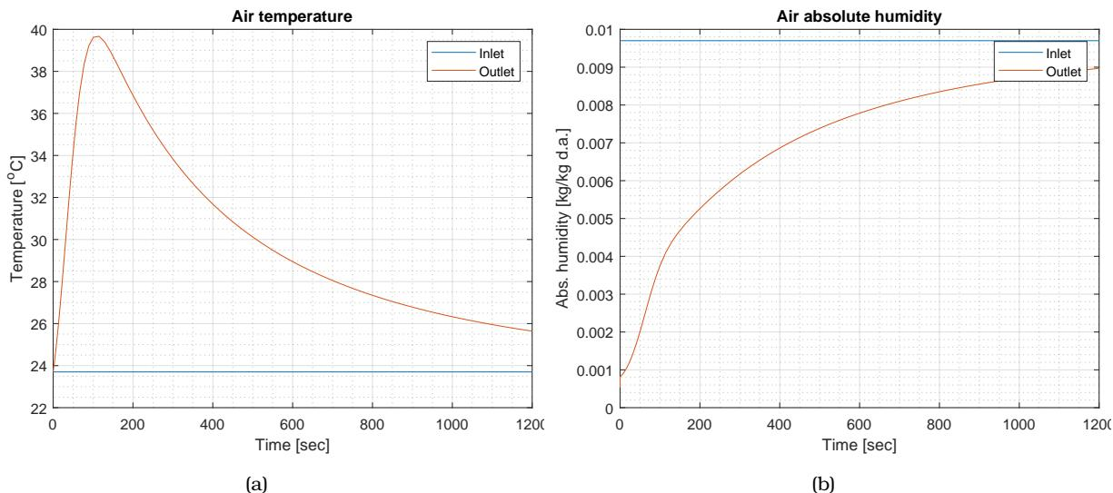
**Figure 2.17:** PGC model results for (a) air temperature and (b) absolute air humidity.
