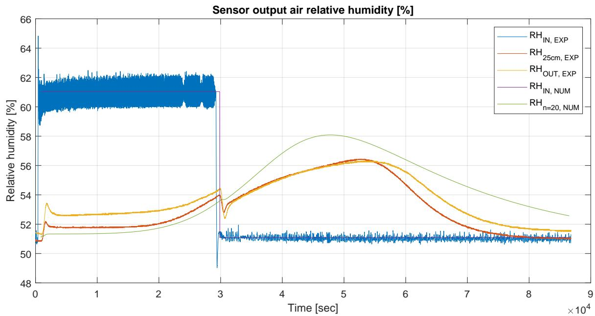
Figure 3.28: Comparison of experimental and numerical results for inlet and outlet relative air humidity.
