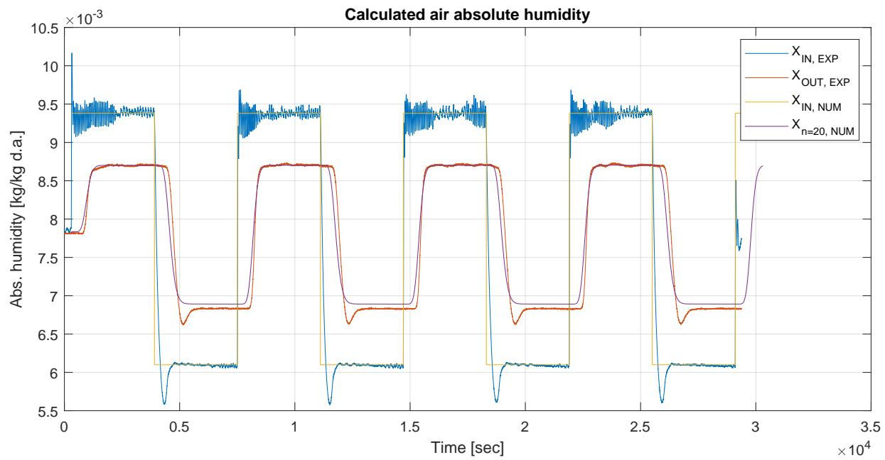
Figure 3.5: Comparison of experimental and numerical results for inlet and outlet absolute air humidity.
