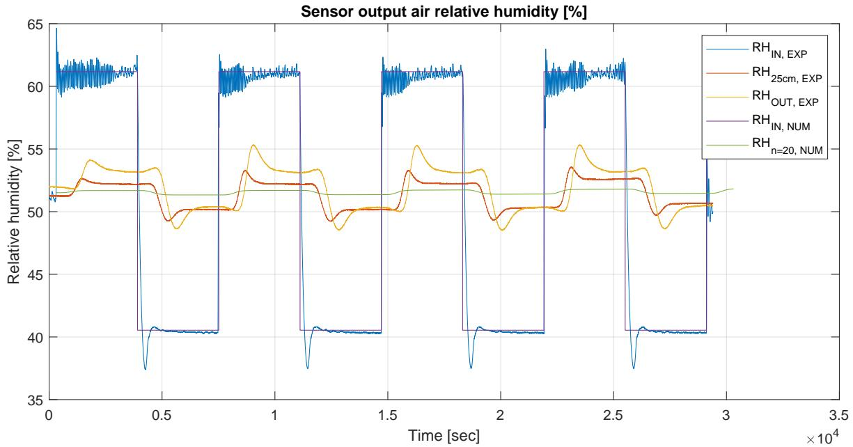
Figure 3.7: Comparison of experimental and numerical results for inlet and outlet relative air humidity.
