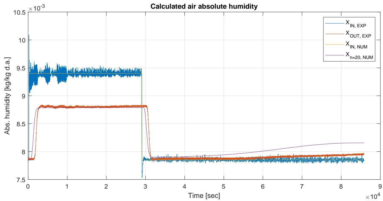
Figure 3.17: Comparison of experimental and numerical results for inlet and outlet absolute air humidity.
