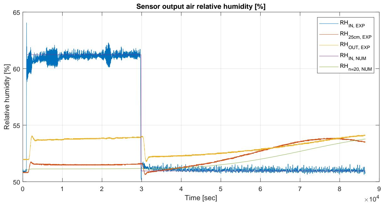
Figure 3.34: Comparison of experimental and numerical results for inlet and outlet relative air humidity.
