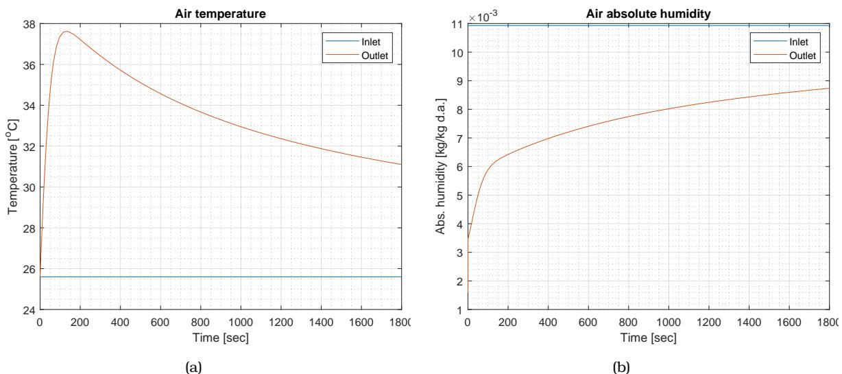
Figure 2.13: PGC model results for (a) air temperature and (b) absolute air humidity.
