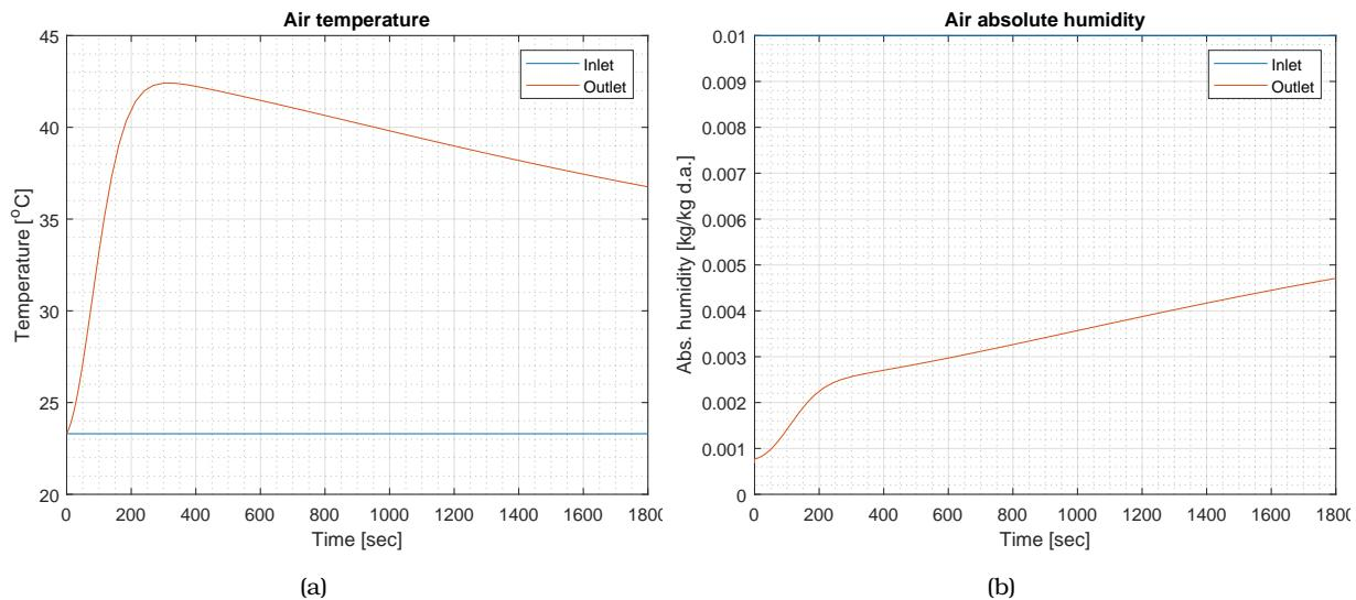
**Figure 2.7:** PGC model results for (a) air temperature and (b) absolute air humidity.
