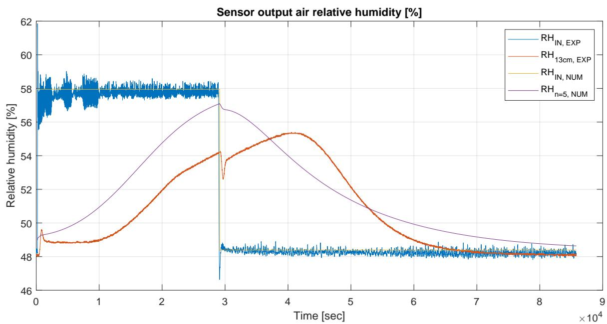
Figure 3.13: Comparison of experimental and numerical results for relative air humidity at 13 cm and  $n = 5$ .
