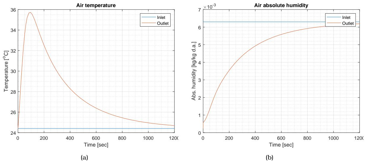
**Figure 2.15:** PGC model results for (a) air temperature and (b) absolute air humidity.
