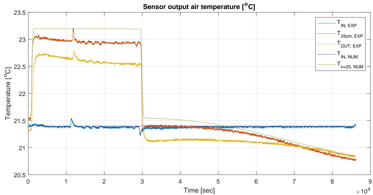
Figure 3.24: Comparison of experimental and numerical results for inlet and outlet air temperature.
