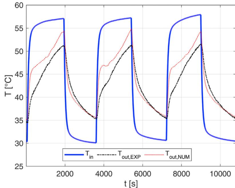
Figure 1.2: Experimental and numerical results for outlet air temperature, after cyclic input to a packed bed, by Antonellis (2019).
