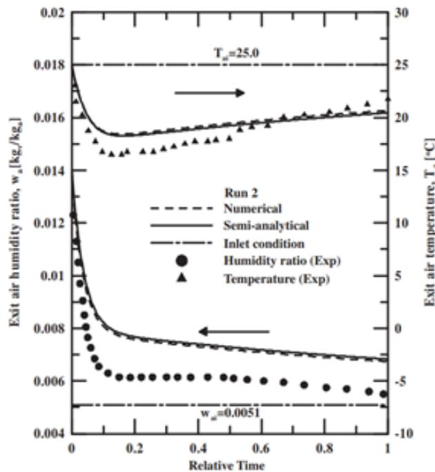
**Fig. 10.** Comparison of the time history of exit air humidity ratio and temperature for Run (2) obtained using semi-analytical, numerical and experimental techniques.
