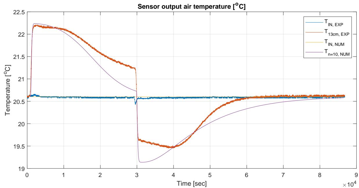
Figure 3.27: Comparison of experimental and numerical results for air temperature at 13 cm and  $n = 10$ .
