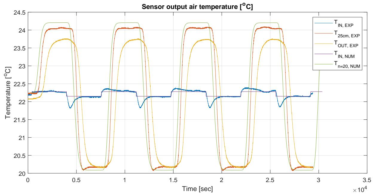
Figure 3.12: Comparison of experimental and numerical results for inlet and outlet air temperature.
