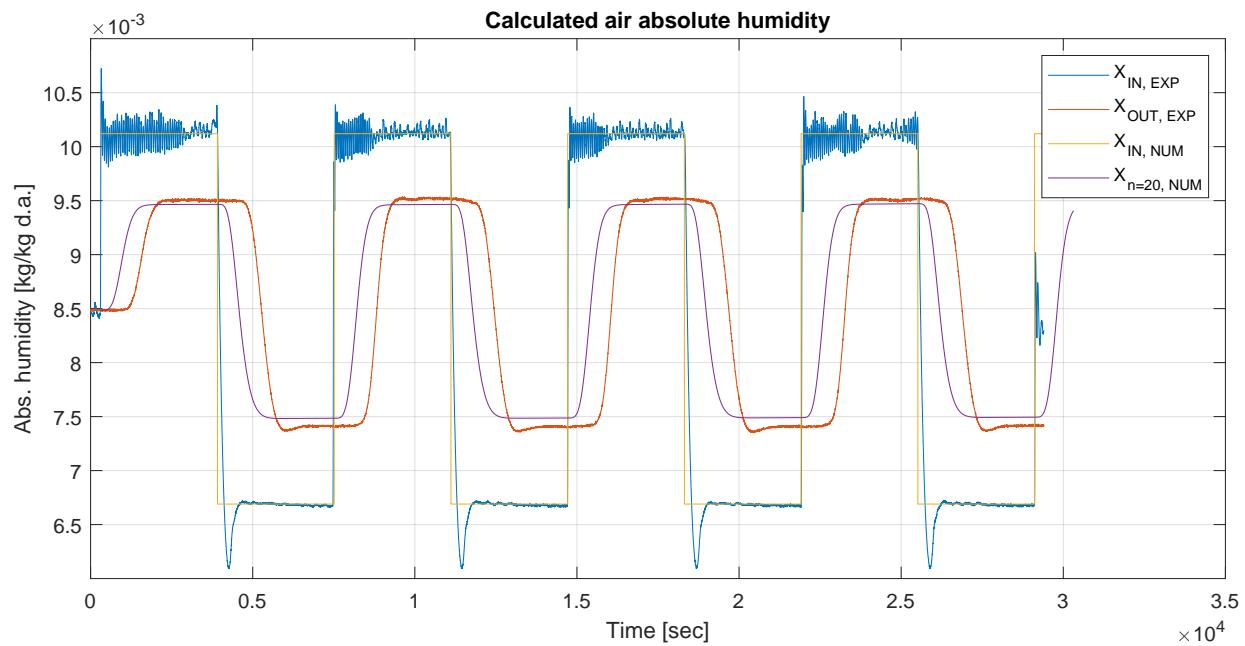
Figure 3.8: Comparison of experimental and numerical results for inlet and outlet absolute air humidity.
