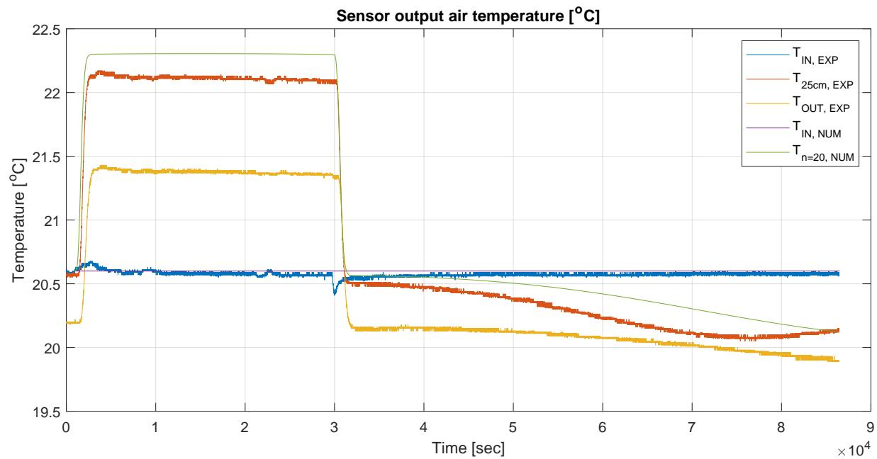
Figure 3.36: Comparison of experimental and numerical results for inlet and outlet air temperature.
