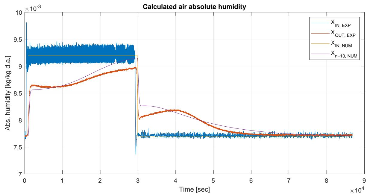
Figure 3.26: Comparison of experimental and numerical results for absolute air humidity at 13 cm and  $n = 10$ .
