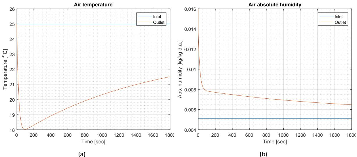
**Figure 2.5:** PGC model results for (a) air temperature and (b) absolute air humidity.
