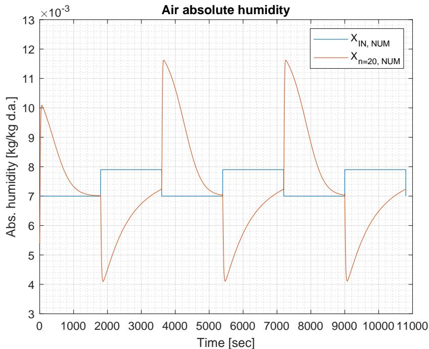
Figure 1.3: Numerical results of PGC model for outlet air absolute humidity, for Antonellis' idealized experimental input
