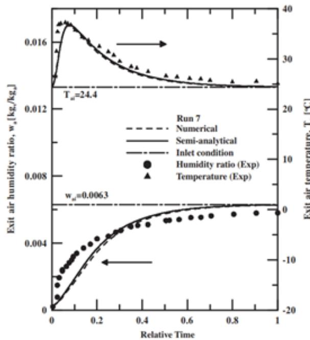
**Fig. 7.** Comparison of the time history of exit air humidity ratio and temperature for Run (7) obtained using semi-analytical, numerical and experimental procedures.
