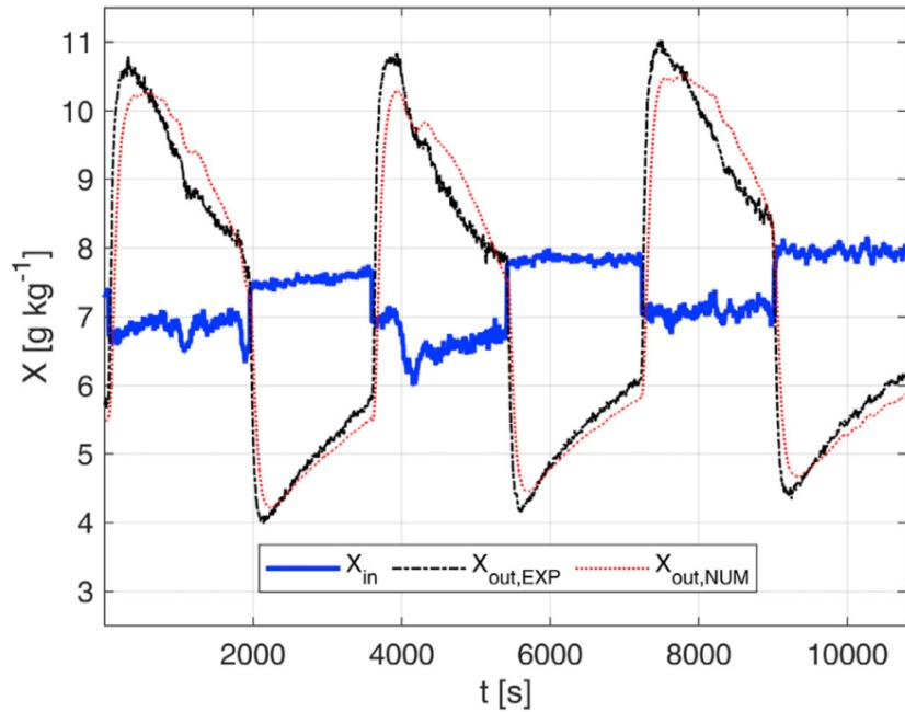
Figure 1.1: Experimental and numerical results for outlet air absolute humidity, after cyclic input to a packed bed, by Antonellis (2019).
