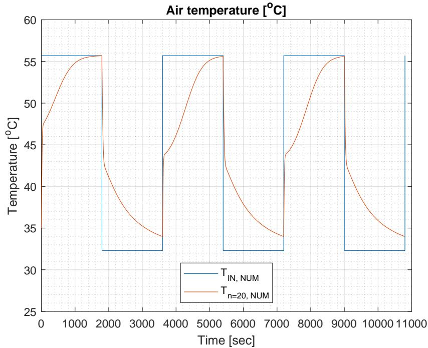
Figure 1.4: Numerical results of PGC model for outlet air temperature, for Antonellis' idealized experimental input
