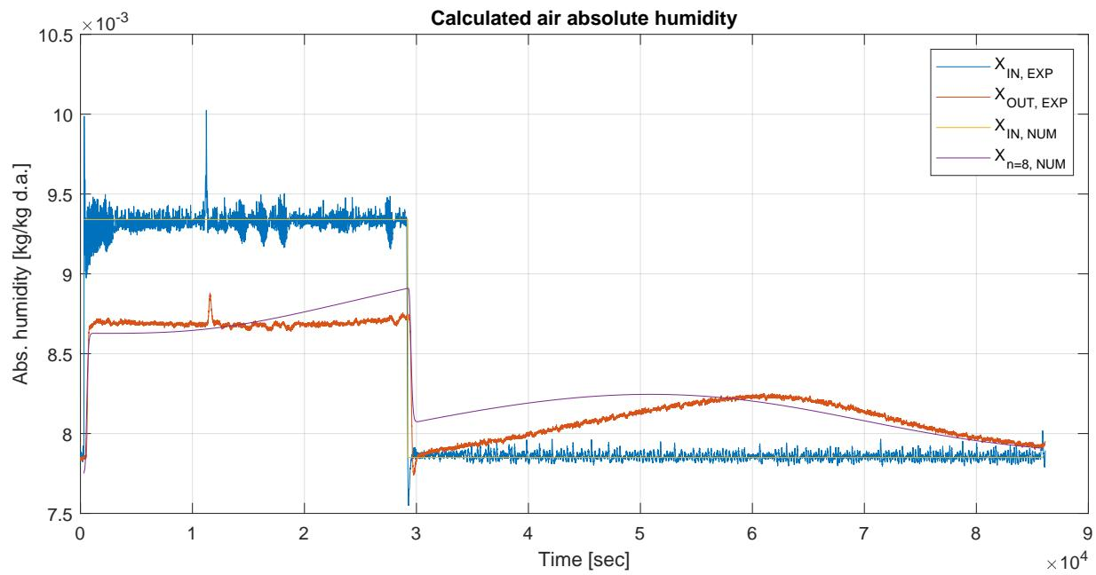
Figure 3.20: Comparison of experimental and numerical results for absolute air humidity at 13 cm and  $n = 8$ .
