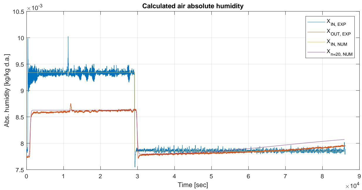
Figure 3.23: Comparison of experimental and numerical results for inlet and outlet absolute air humidity.
