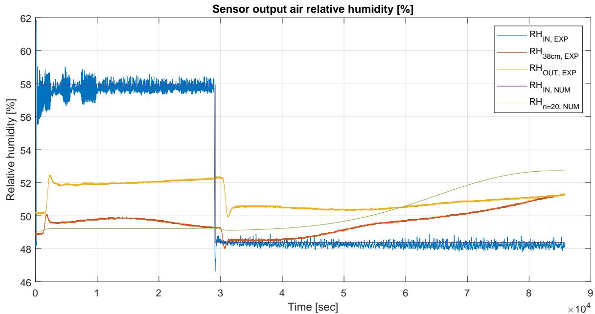
Figure 3.16: Comparison of experimental and numerical results for inlet and outlet relative air humidity.
