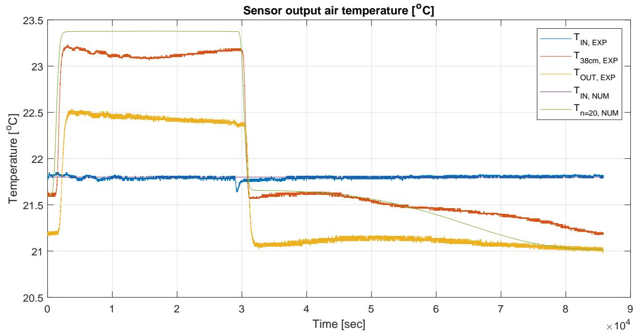
Figure 3.18: Comparison of experimental and numerical results for inlet and outlet air temperature.
