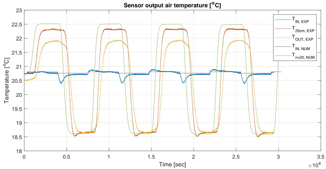
Figure 3.3: Comparison of experimental and numerical results for inlet and outlet air temperature.
