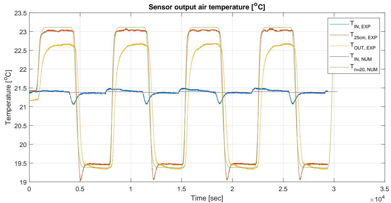
Figure 3.6: Comparison of experimental and numerical results for inlet and outlet air temperature.
