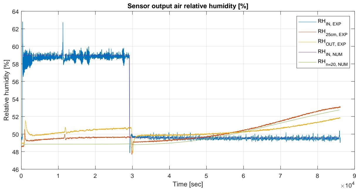
Figure 3.22: Comparison of experimental and numerical results for inlet and outlet relative air humidity.
