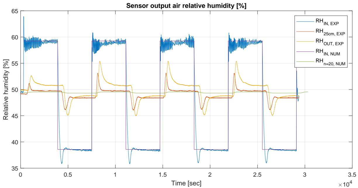
Figure 3.4: Comparison of experimental and numerical results for inlet and outlet relative air humidity.
