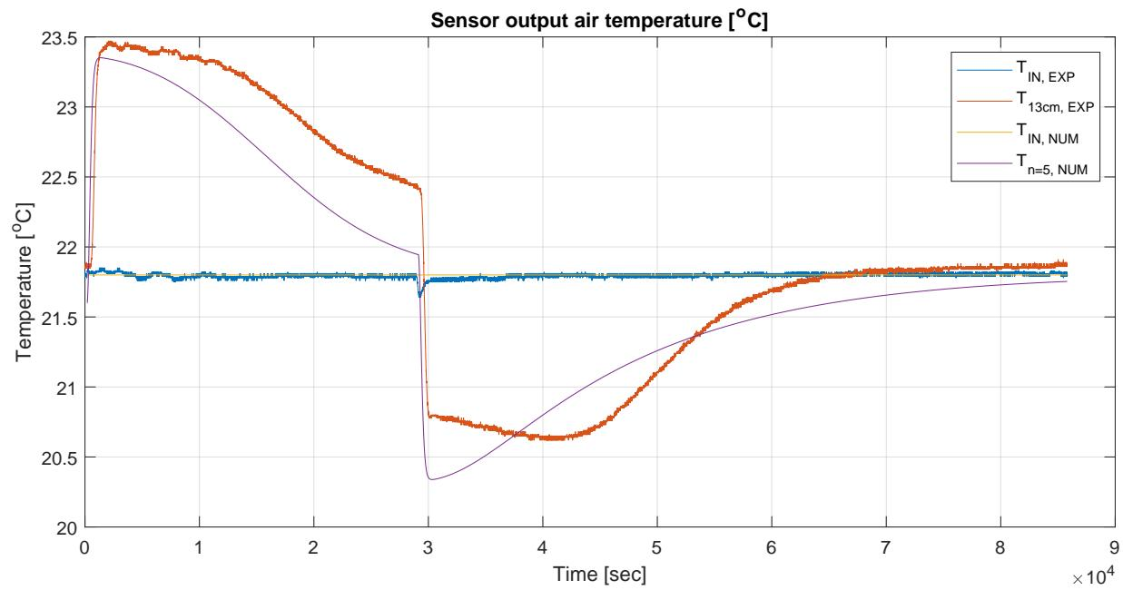
Figure 3.15: Comparison of experimental and numerical results for air temperature at 13 cm and  $n = 5$ .
