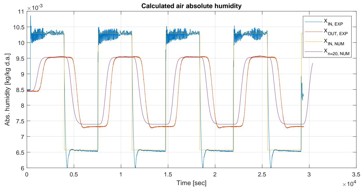
Figure 3.11: Comparison of experimental and numerical results for inlet and outlet absolute air humidity.
