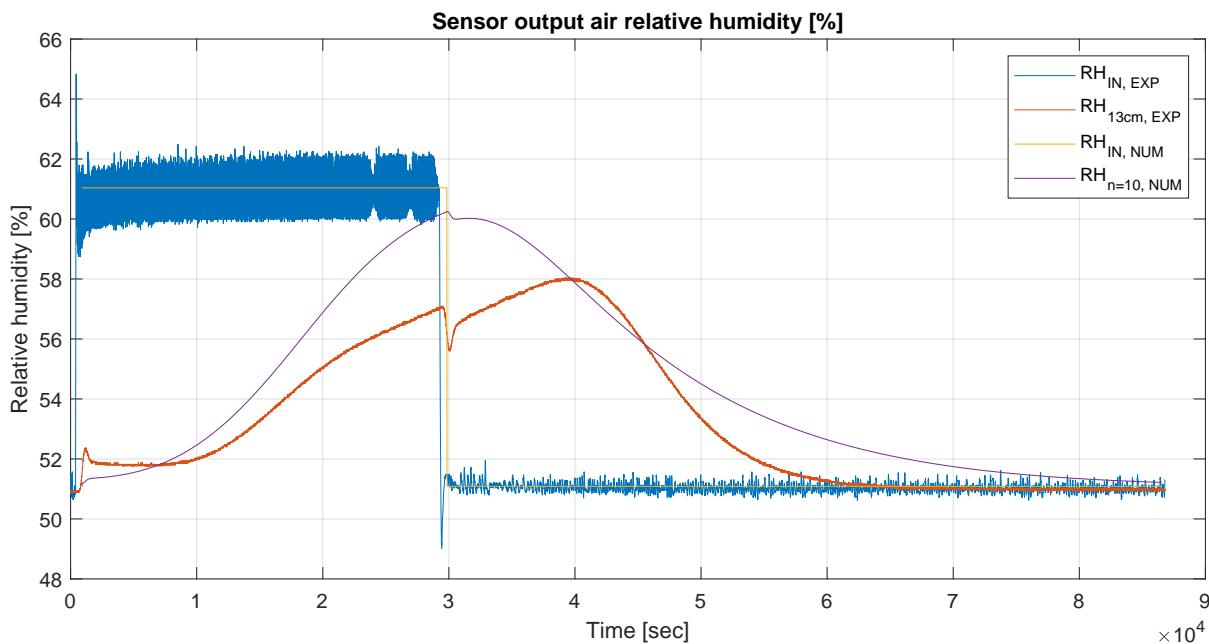
Figure 3.25: Comparison of experimental and numerical results for relative air humidity at 13 cm and  $n = 10$ .
