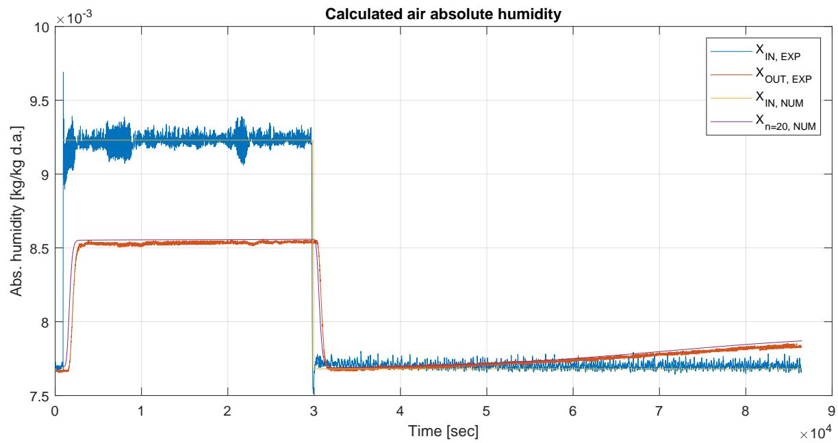
Figure 3.35: Comparison of experimental and numerical results for inlet and outlet absolute air humidity.
