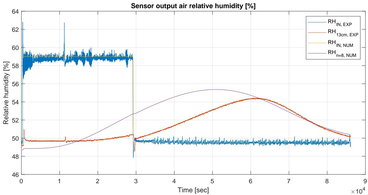
Figure 3.19: Comparison of experimental and numerical results for relative air humidity at 13 cm and  $n = 8$ .
