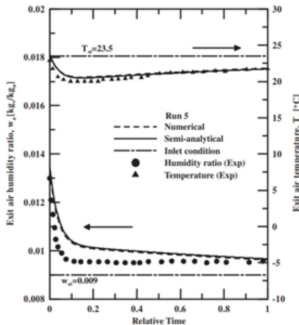
**Fig. 11.** Comparison of the time history of exit air humidity ratio and temperature for Run (5) obtained using semi-analytical, numerical and experimental techniques.
