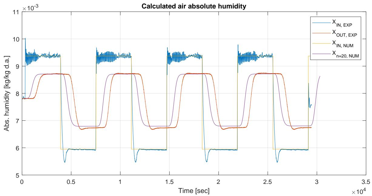
Figure 3.2: Comparison of experimental and numerical results for inlet and outlet absolute air humidity.
