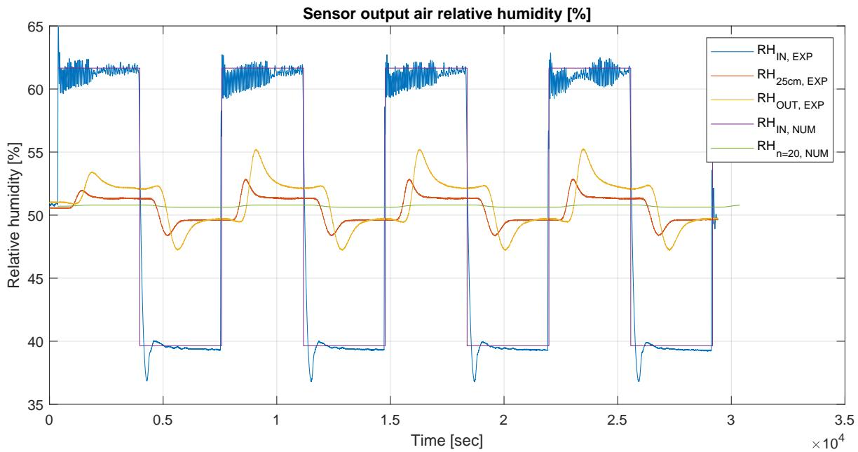
Figure 3.10: Comparison of experimental and numerical results for inlet and outlet relative air humidity.
