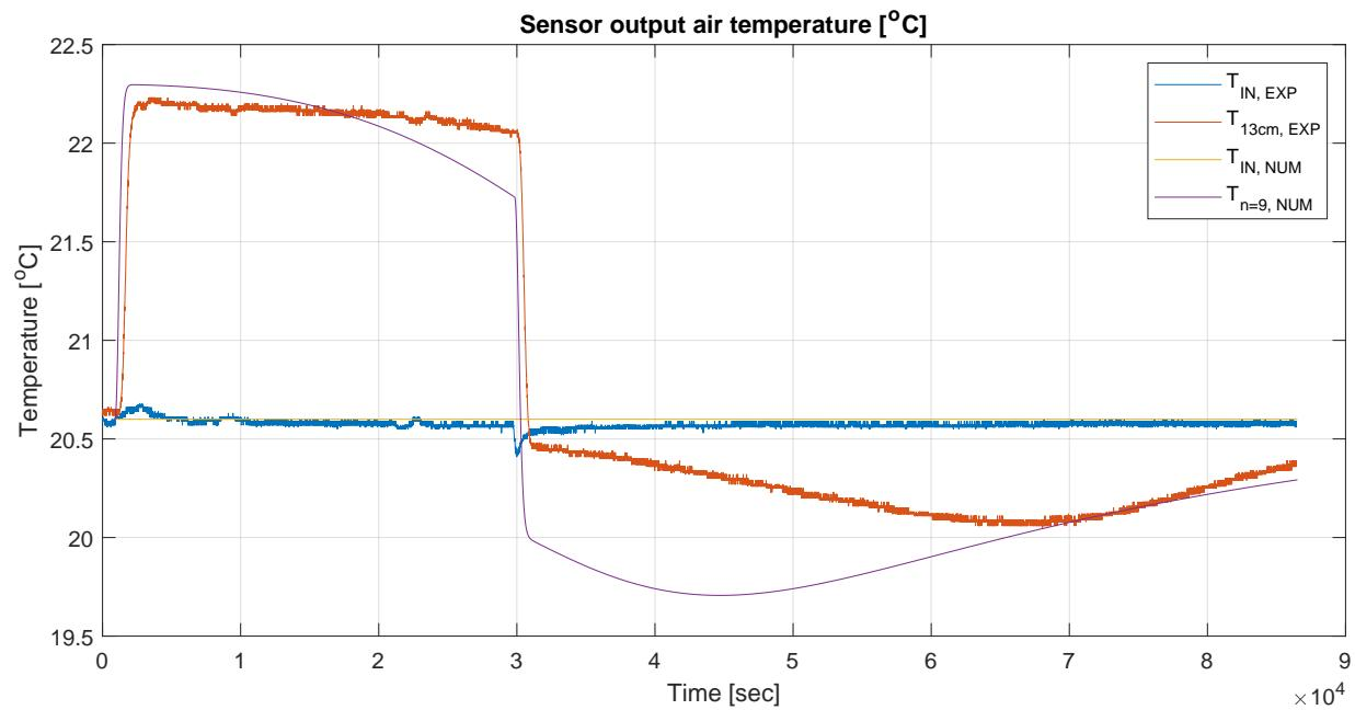
Figure 3.33: Comparison of experimental and numerical results for air temperature at 13 cm and  $n = 9$ .
