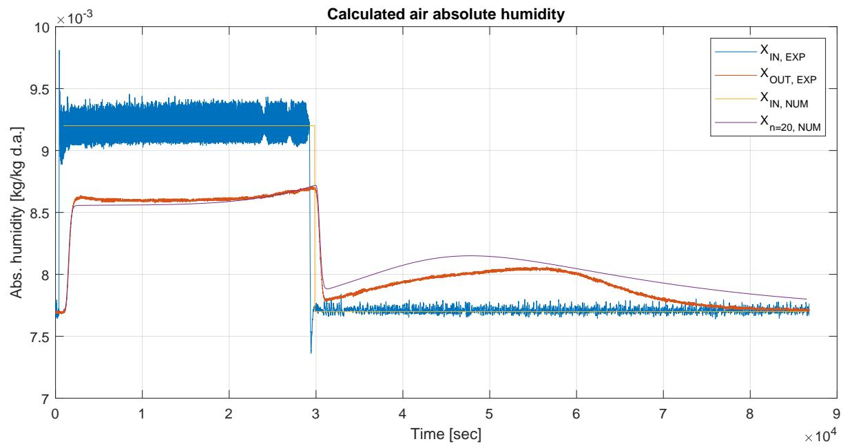
Figure 3.29: Comparison of experimental and numerical results for inlet and outlet absolute air humidity.
