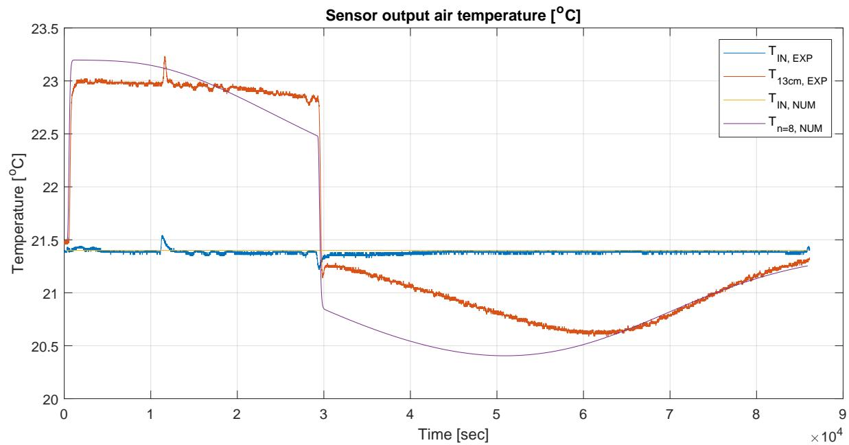
Figure 3.21: Comparison of experimental and numerical results for air temperature at 13 cm and  $n = 8$ .
