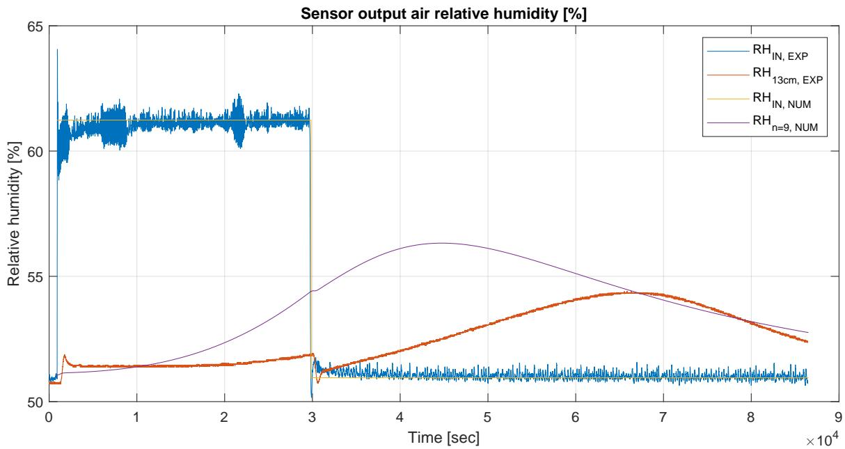
Figure 3.31: Comparison of experimental and numerical results for relative air humidity at 13 cm and  $n = 9$ .
