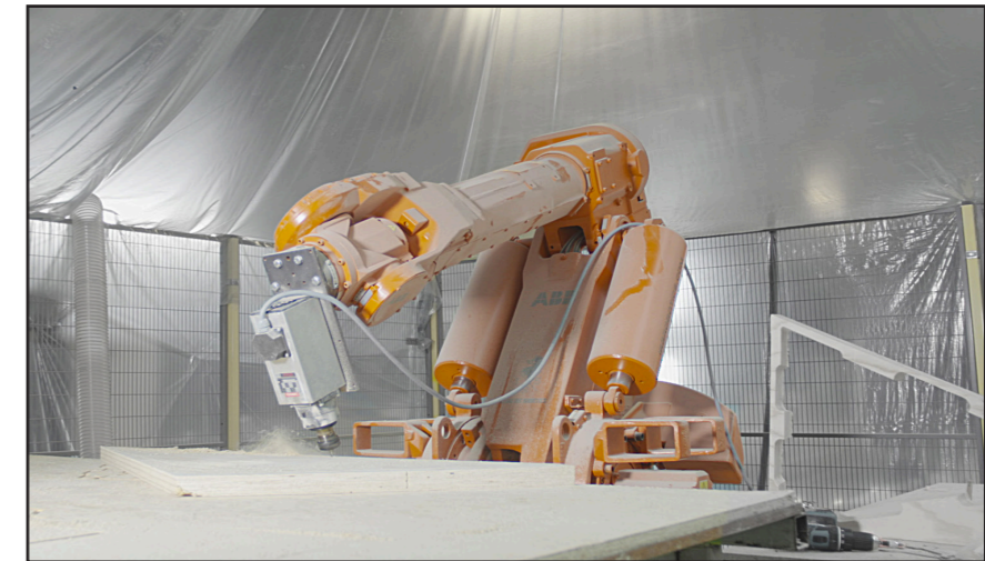
all parts are planar and can be cut out of a sheet of plywood using CNC-technology.
