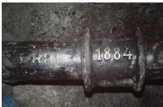
Figure 7.9: Example of an old CI pipe from 1884 recently removed in Schiedam [59]
