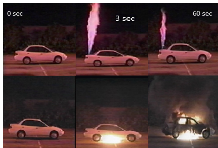
Figure 3.3: Comparison between a hydrogen (top) and gasoline (bottom) fire in a car
