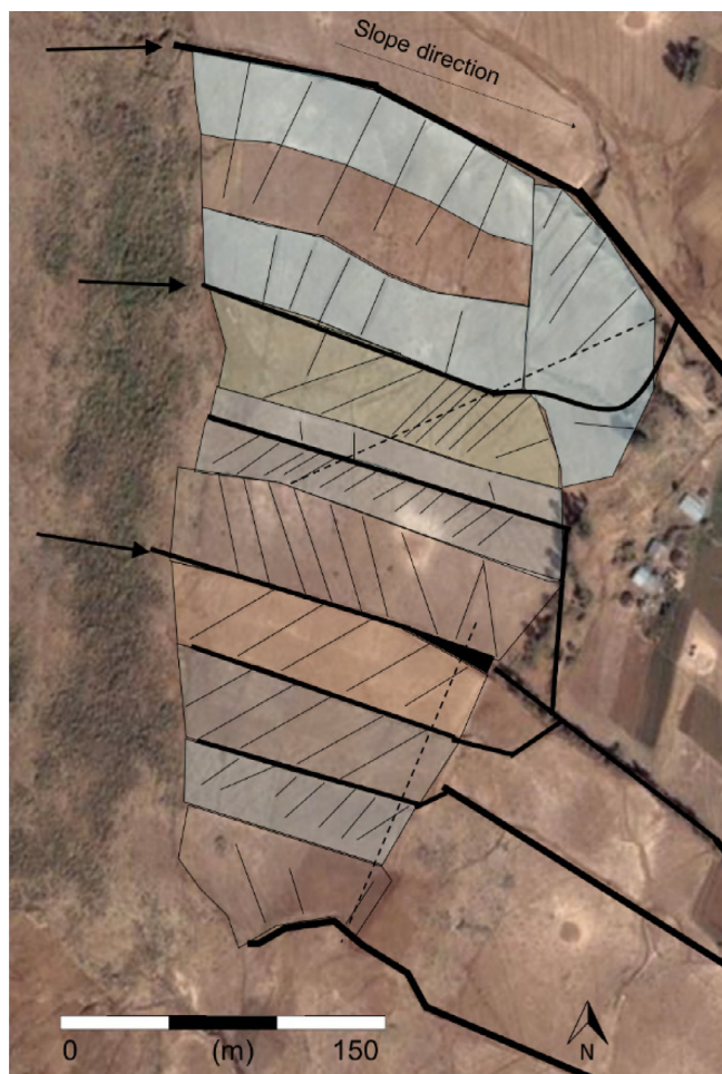
Figure 7. Detail of pattern of furrows (thin lines) and drains (bold lines) above Abebe's house (see Figure 2). Note: The furrows of all but one plot end in "vertical" drains that direct the water straight down the slope. The two dashed lines indicate the remains of two drains dating back to the Dergue period (1974–91).
