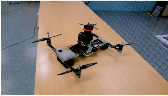
Figure 2. Quadrotor developed at ISIR, equipped with a Hokuyo URG-30LX 2D LiDAR, an MPU6000 3 axis accelerometer/gyrometer unit and an SF10/A laser altimeter from Lightware Optoelectronics.
