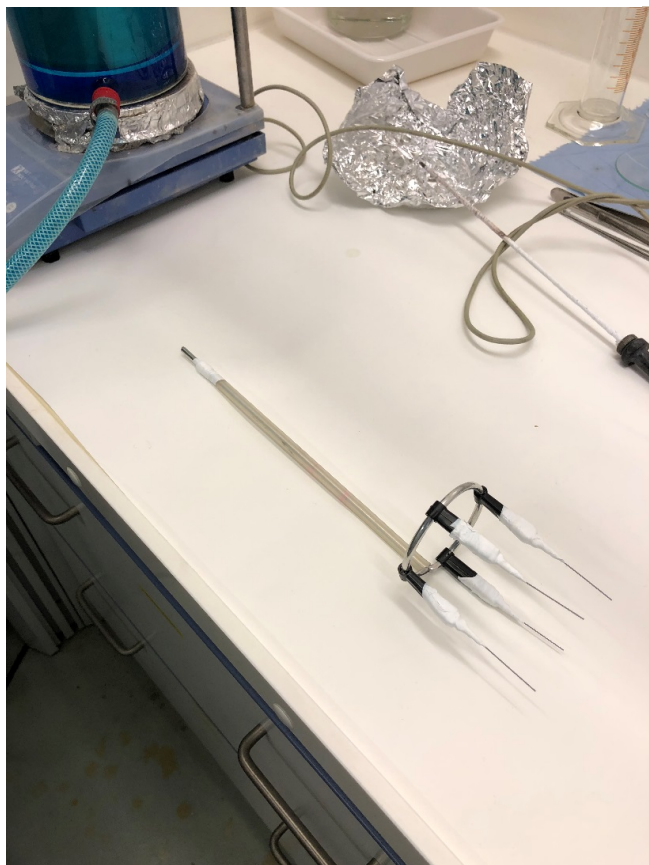
Figure 15 Multi holder with implants. a) showing the finished multi holder, with four implants isolated using isolation tape. b) the multi holder positioned in the centre of the electrolytic cell, indicated by the vortex as result of the stirring of the electrolyte.
