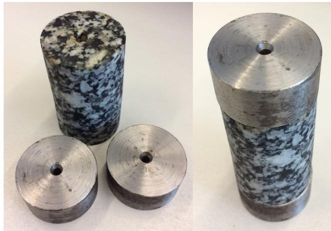
*Fig 2.1: Rock sample with a drilled hole in the middle and steel cylinders placed on top and bottom of the specimen during Experiments 8 and 9. Prepared rock samples for the fracture Experiments 1 – 5 are identical except the drilled hole.*
