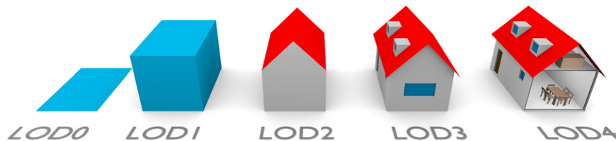
Figure 2.2.: Illustration of a single building in different LoD. Figure retrieved from Biljecki et al. [2016]
