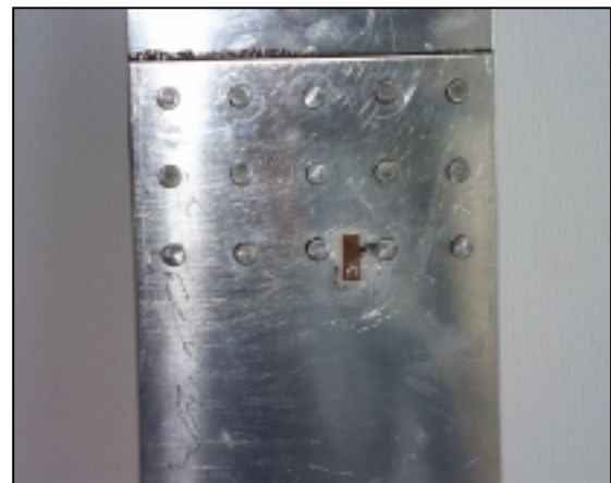
Figure 10.5. 2024T3 lap joint specimen with attached strain gauges
