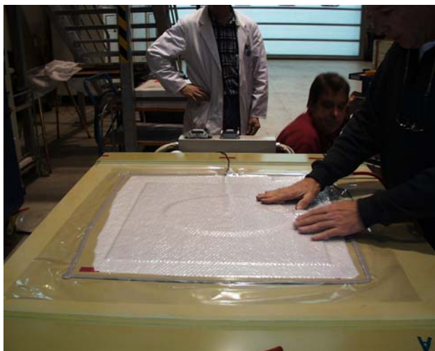
Application of vacuum foil, thereafter start of curing with Heatcom ® device, low vacuum pressure (for specimens 12-BR-1 and 12-BR-2)
