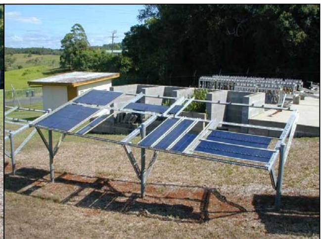
Figure 3.4.3. Exposure rack carrying different specimen types
