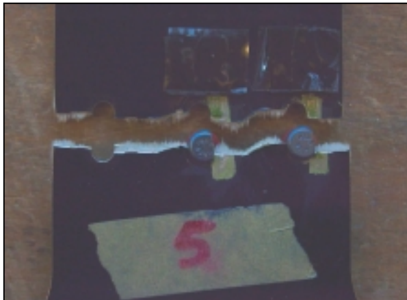
Figure 6.9.2. Milled specimen, shown after failure
