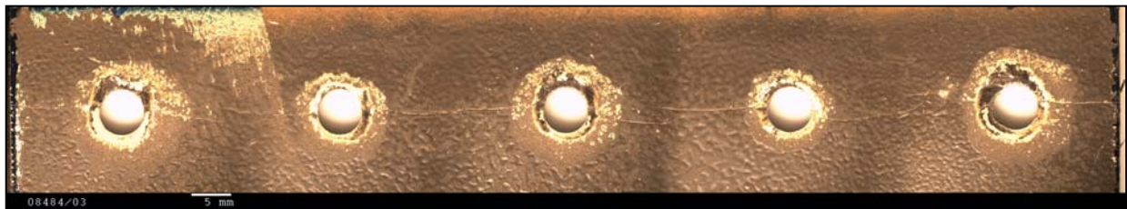
Figure 7.1.8.25. View on specimen 2-A-48, rivet row 1, mating aluminium layer
