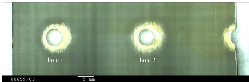
Figure 7.1.8.26. View on prepeg below free metal surface, prepeg damages around all holes
