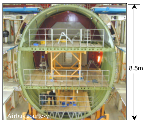
Figure 3.1.2. View on cross section of Airbus ‘Megaliner Barrel’, details on following pages
