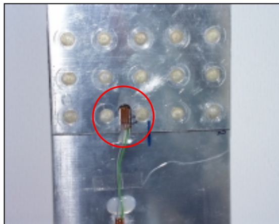
Figure 10.5. 2024T3 lap joint specimen with attached strain gauges
