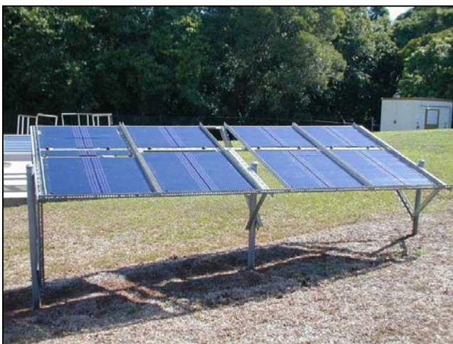
Figure 3.4.2. Exposure rack with 2-B- specimens
