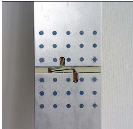
Figure 7.1.2.11. Joint specimen for bending investigations, aluminium skin sheets, GLARE2 butt strap
