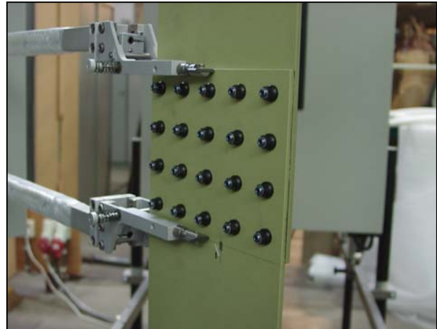
Figure 7.1.7.4. Extensometer positioning on riveted repair coupon, specimen series 2-A
