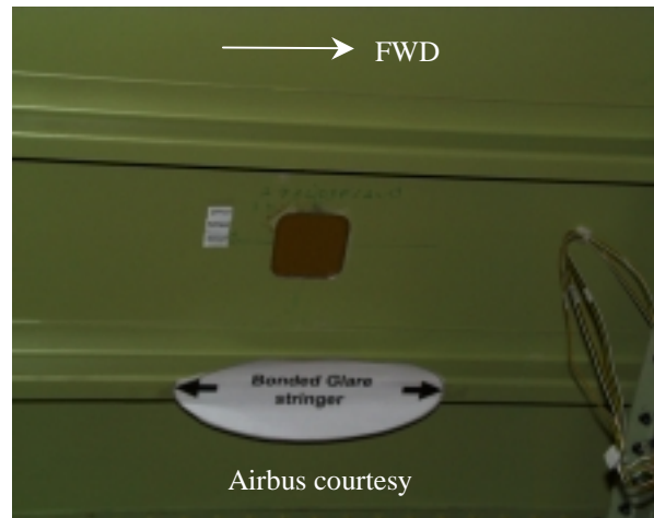
Figure 9.2. Cut out below bonded repair patch, view from inside, between stringer 3 & 4
