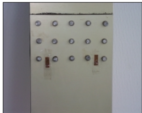
Figure 10.4. GLARE3.5/4-.4 lap joint specimen with attached strain gauges
