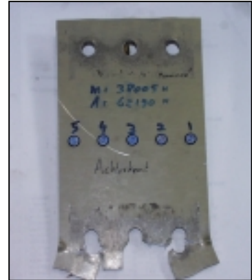
Figure 6.9.1. Specimen 3-B-1 after residual strength test
