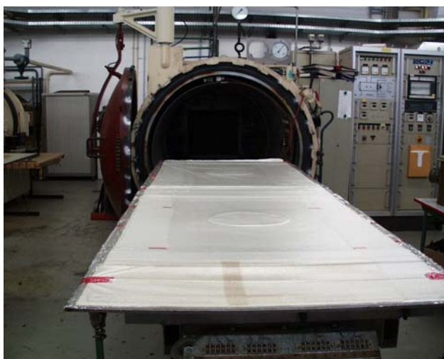
For specimens 12-BR-03 to 12-BR-05: curing in autoclave at 3 bar vacuum pressure
