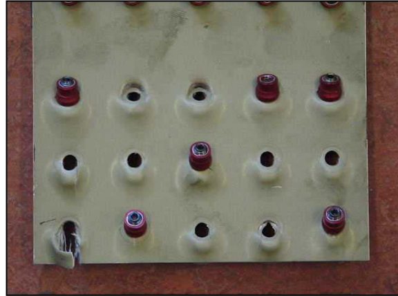
Figure 7.1.8.2b. View on specimen 2-B-88 after failure, butt strap collar side
