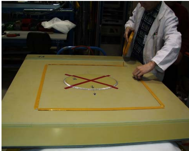
Fixation of GLARE patch in order to avoid movement during curing
