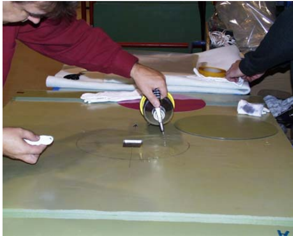
Front side of panel, application of cleaning agent according to Airbus technical instruction 80-T-35-0014
