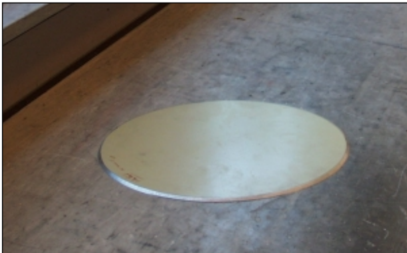
Figure 9.4. Repair doubler for Megaliner Barrel before bending to final shape
