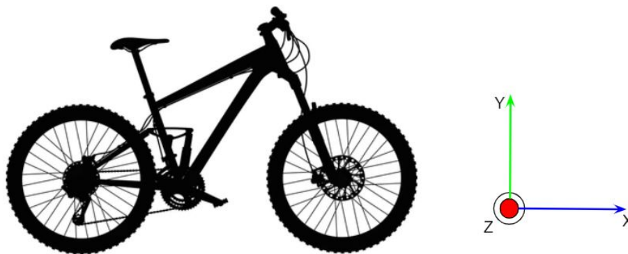
Figure 3.7: The XY plane vibration modes of the bicycle components are referred to as the in-plane vibration modes and the YZ plane vibration modes are referred to as out-of-plane vibration modes for this project
