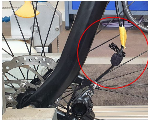
Figure 3.4: Microphone placement near to the frictional interface to capture the brake noise audio data
