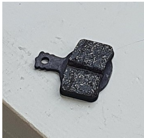
Figure 7.3: 1.5 mm wide and 2 mm deep parallel slot in the friction lining dividing it into two small blocks for better heat conduction
