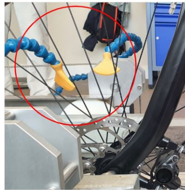
Figure 3.2: Yellow nozzles in the red circle used to spray water onto the rotor and pad interface
