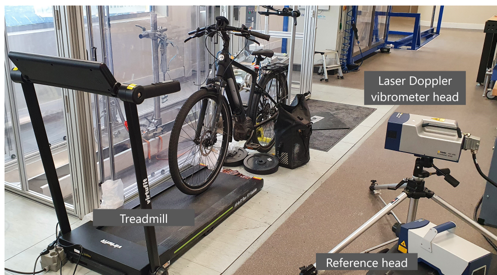
Figure 3.5: Test bench with treadmill to run the bike with an unrestricted view of the rotor for the laser vibrometer to capture the vibration velocity
