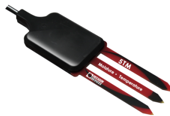
(b) Example of a type of soil moisture sensor: Decagon 5TM watercontent sensor [32]
