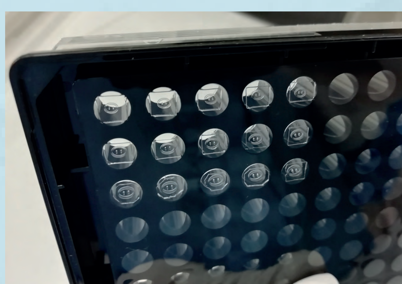
PDMS chips transferred to a 96-well plate for cell culturing experiments
