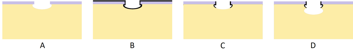
Figure 3.3: A schematic representation of a 3-step DRIE process. Adapted from [54]
