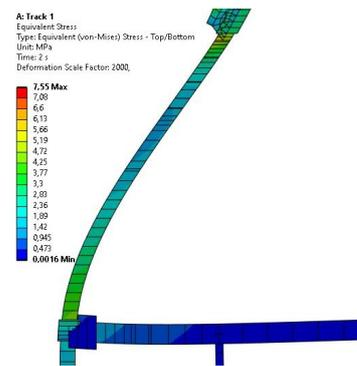
**Figure E.66:** Zoomed in, equivalent stress and deformed shape,  $T_{deck} = 40$  [mm] and  $t = 2$  [s] [3]
