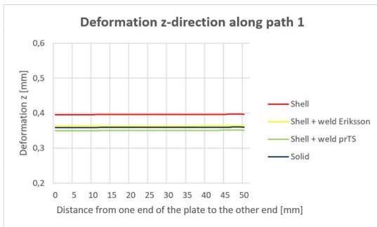
Figure C.19: Transverse fillet weld, out-of-plane torsion deformation Z
