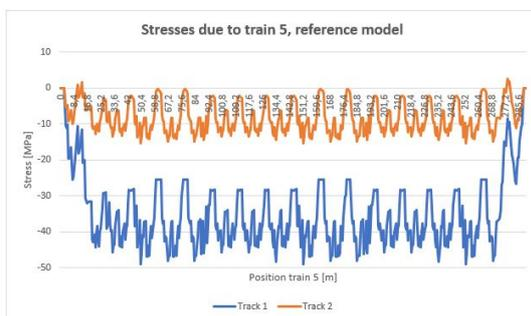
Figure D.7: Train 5, stress plot hand calculation
