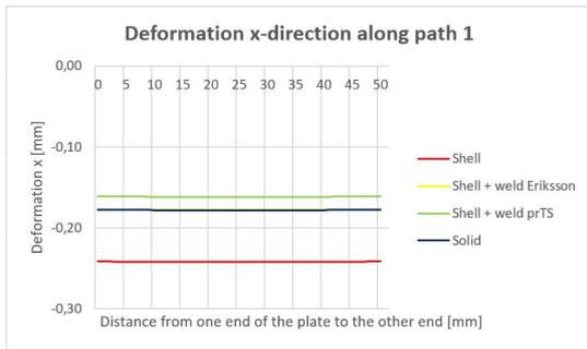
Figure C.11: Transverse fillet weld, in-plane torsion deformation
