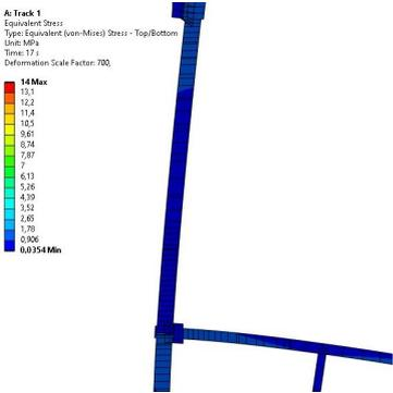
Figure E.61: Zoomed in, equivalent stress and deformed shape,  $T_{dia} = 10 [mm]$  and  $t = 17 [s]$  [3]
