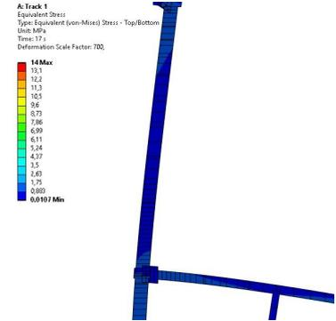
Figure E.62: Zoomed in, equivalent stress and deformed shape,  $T_{dia} = 30 [mm]$  and  $t = 17 [s]$  [3]
