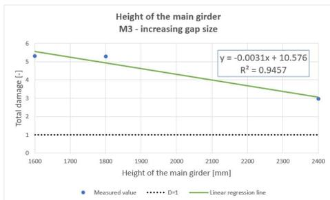
**Figure F.7:** Linear regression detail M3:  $H_{mg}$
