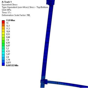
Figure E.42: Zoomed in, equivalent stress and deformed shape,  $H_{mg} = 2400 [mm]$  and  $t = 17 [s]$  [3]
