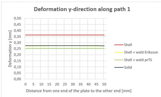
Figure C.7: Transverse fillet weld, in-plane bending deformation
