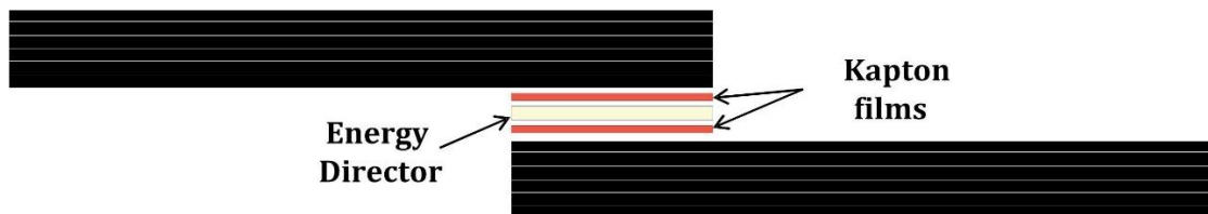
Figure 3.6. Schematic of specimen prepared for removing the energy directors from the weldline in order to perform direct crystallinity measurements. Dimensions are not to scale.
