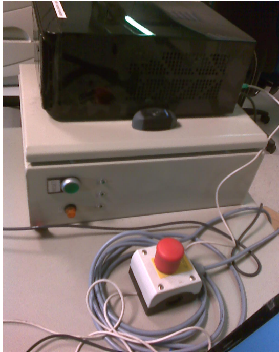
Figure 2: Original computer and Power controller with red Emergency stop button
