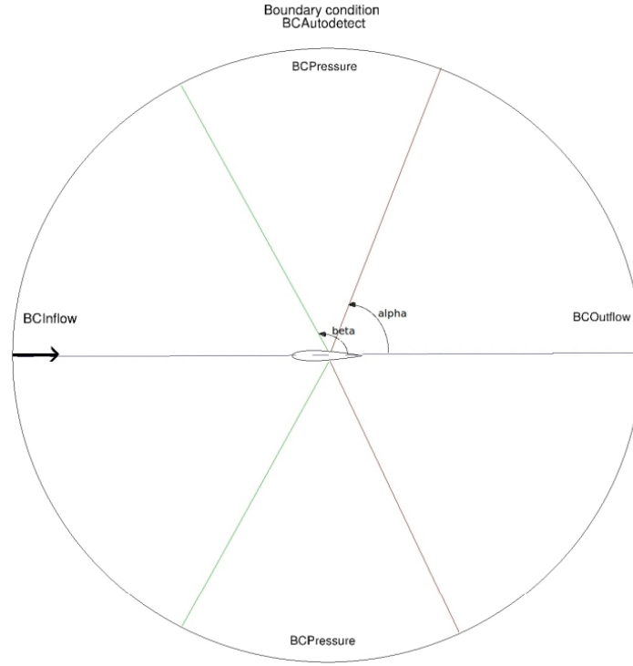
Figure 4-4: Geometry of the autodetect boundary conditions [67].
