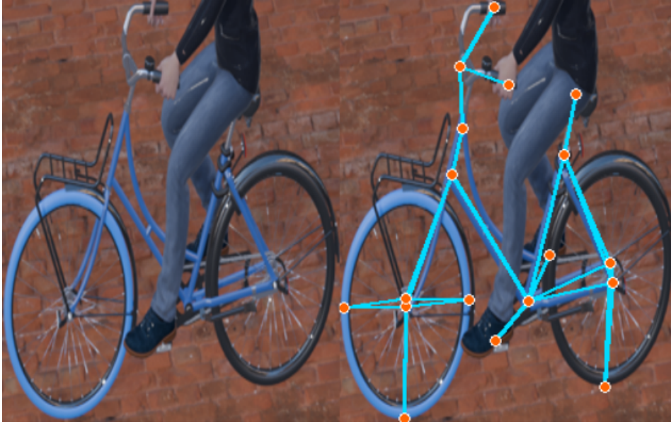
Figure 3.7: RTMPose-L input and output for a single frame: the bicycle image (left) and the predicted two-dimensional keypoints with the bicycle skeleton (right).
