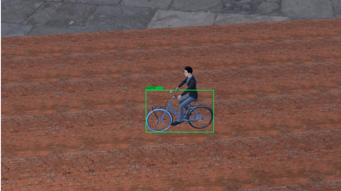
Figure 3.6: The result of RF-DETR detecting a bicycle with 91% confidence.
