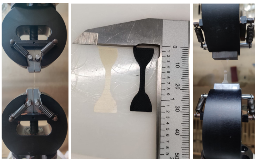
Figure 6.4: Clamp holding the polymer samples (left), Dumbbell-shaped samples (middle), and a proper fracture at the middle of the polymer (right)
