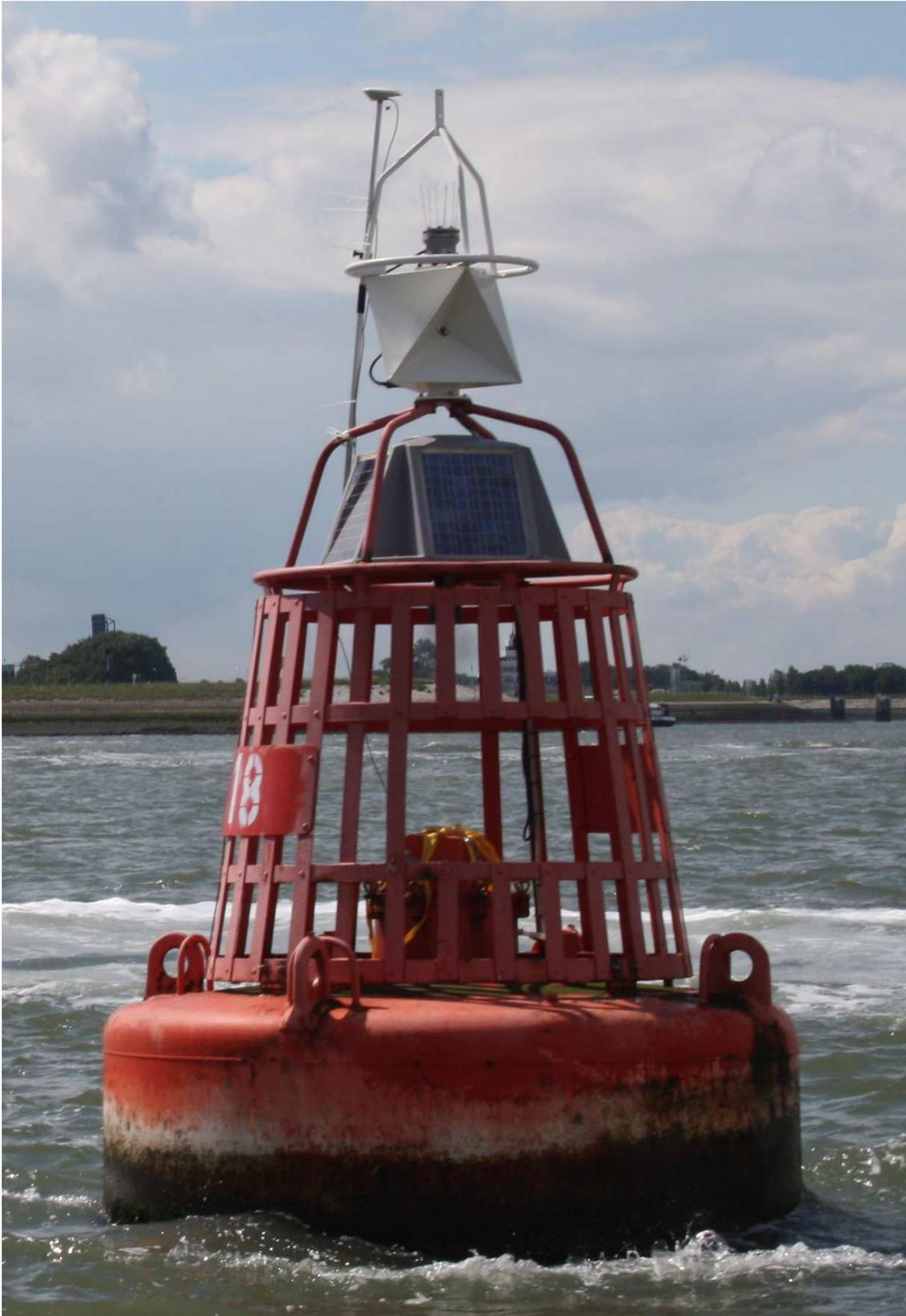
**Figure 3.8:** Buoy 18 is located near Terneuzen. For this buoy the Trimble R7 GPS receiver is mounted inside the cage. The Trimble Zephyr antenna is installed on a range pole on top of the buoy. Note the eddies induced by the tidal current around the buoy.
