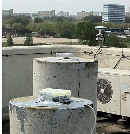
**Figure 3.6:** Measurement set-up on the NMi roof, the Septentrio AsteRx1, the Vincotech 1084A and the Garmin are set-up at different marker locations.
