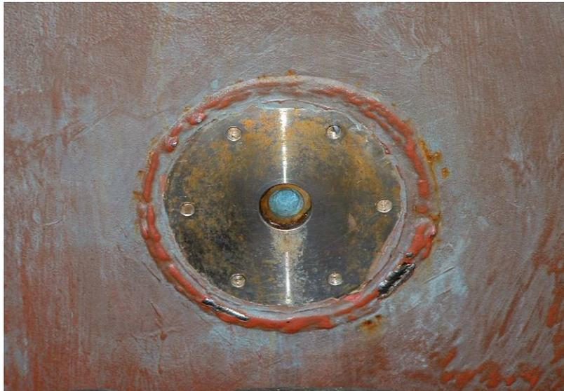
Figure B.2 Wave pressure sensor fitted on Glas Dowr
