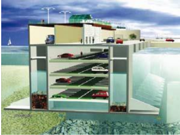
Figure 8: Pier extension floating breakwater in Monaco 8
