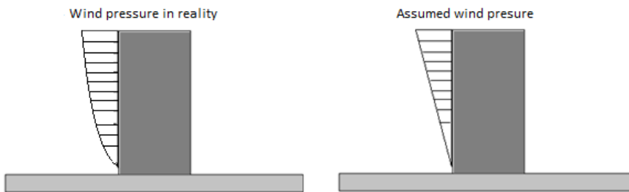
Figure 42: Wind load in reality versus assumption of the wind load acting on a building
