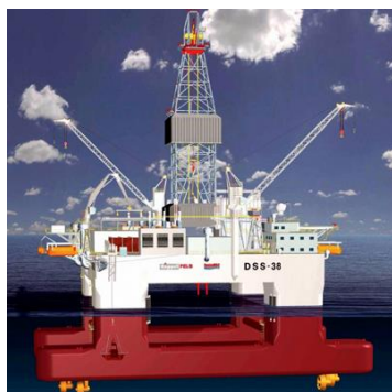
Figure 21: Column-stabilized semi-submersible structure 13
