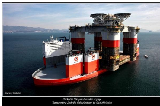
Figure 20: Ship transporting a bottle-type semi-submersible 12
