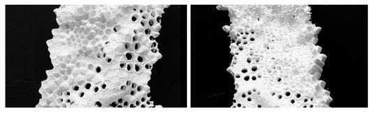
FIGURE 5 Porous Assembly: Exterior (left) and interior (right) sides
