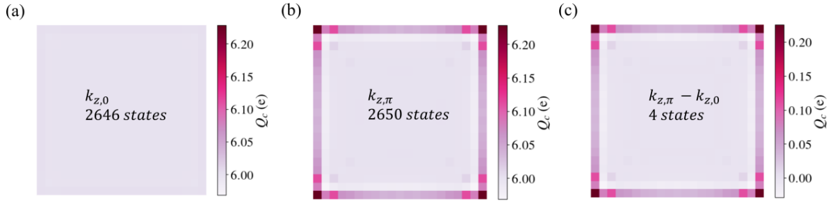
Figure A.2: (a) Probability density of all occupied bulk states at k_z = 0 for a 21 \times 21 (100) nanowire. (b) Probability density at k_z = \pi/a including four gapless states crossing the Fermi level. (c) Difference between plot (b) and (a), revealing the corner charge.
