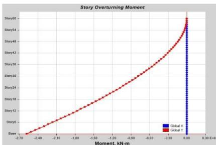
FIG 6.71. Overturning moment, beam model
