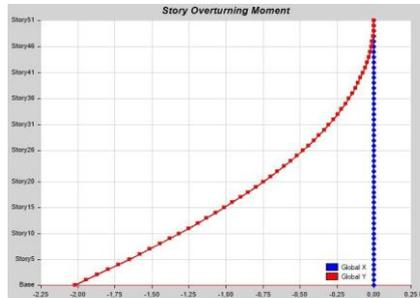
FIG 6.64. Moment, walls with beam mech prop
