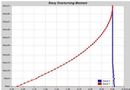
FIG 6.63. Overturning moment, beam model
