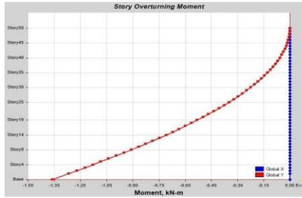
FIG 6.35. Moment, walls with beam mech prop
