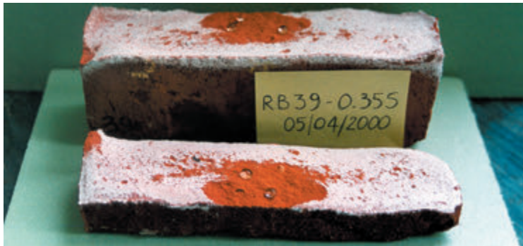
Figure 6: Spalling of a salt loaded brick treated with a water repellent
