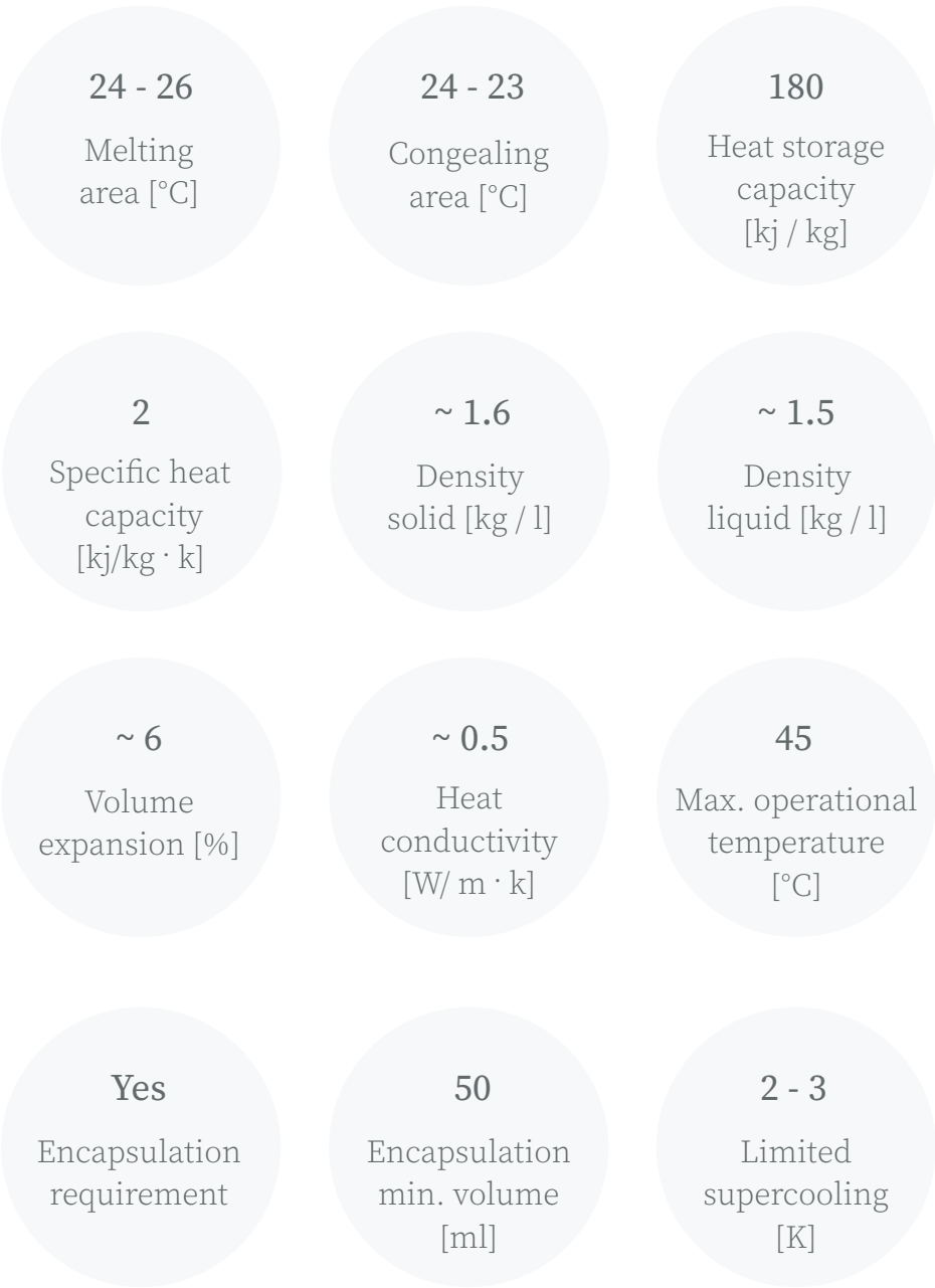
Figure 3.9: properties of chosen PCM (technical sheet in Appendix) Source: edited from SP25E2, by Rubitherm, n.d., http://bit.ly/3w-QiNDW
