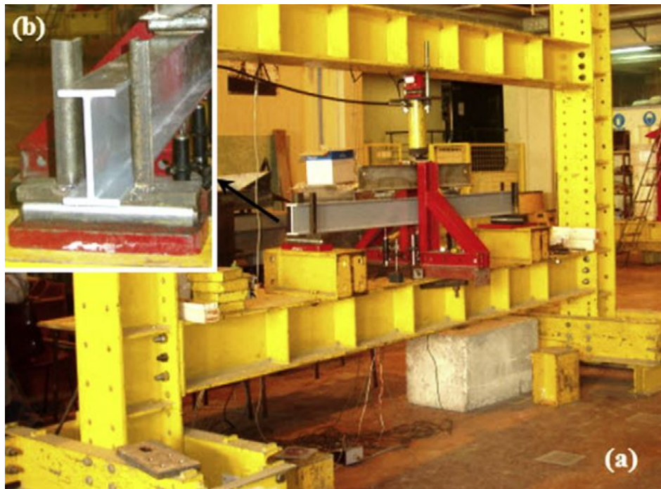
Figure 3-1: Four point bending creep test setup [9]
