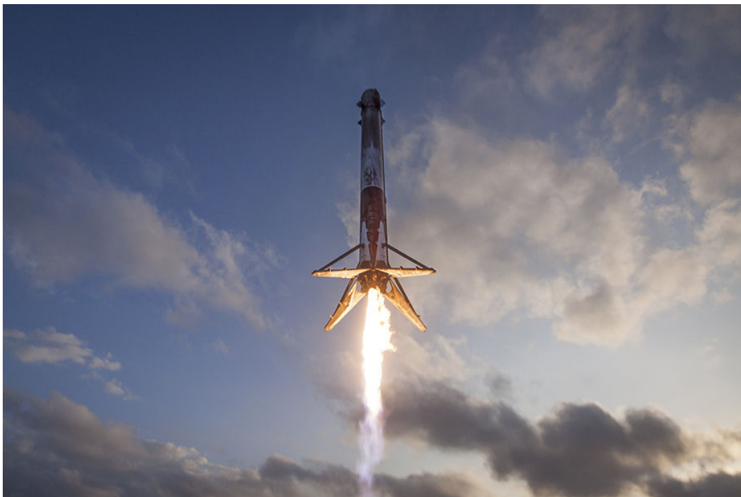
Figure 2.3: Close-up of a Falcon 9 landing burn with landings legs deployed [19].
