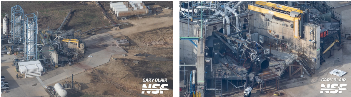
Figure 2.5: SpaceX McGregor horizontal test stand: (left) Full test bench with LOX and CH 4 tanks clearly visible; (right) Test cell with Raptor 3 [86].
