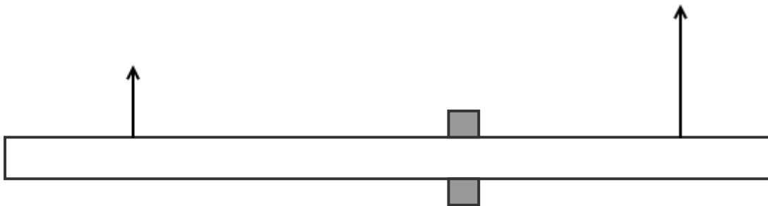
Figure 10.5: Fuselage cantilever beam model
