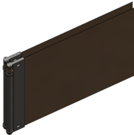
Figure 2.11: Illustration of the pulling concept, where at the tip small motors provide the actuation of the finger.
