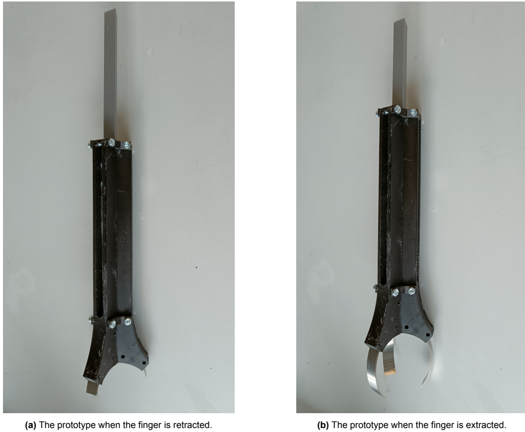
Figure 9.3: A picture of the final prototype in retracted and extracted configuration.
