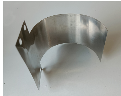
(b) The stainless steel testpiece, laser cut and curved.
