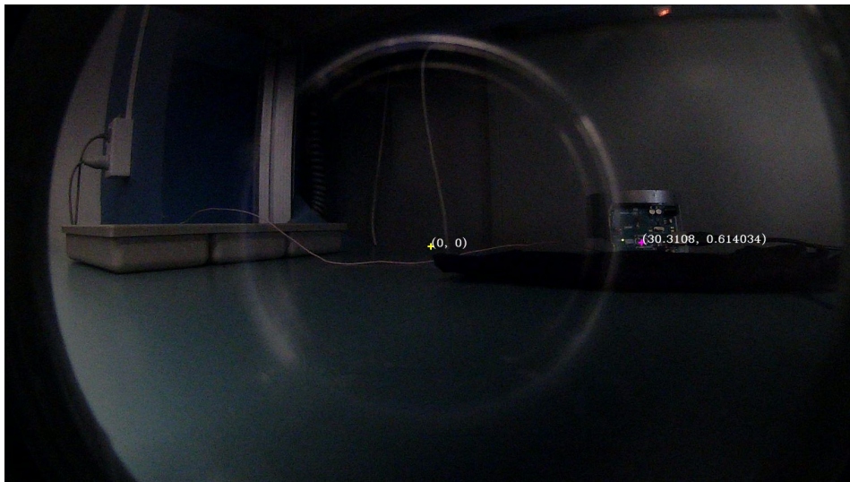
Figure 4.10: Example of test showing the determination of the spherical coordinates with respect to the camera. The LED in this situation is located 30 degrees to the right of the camera.
