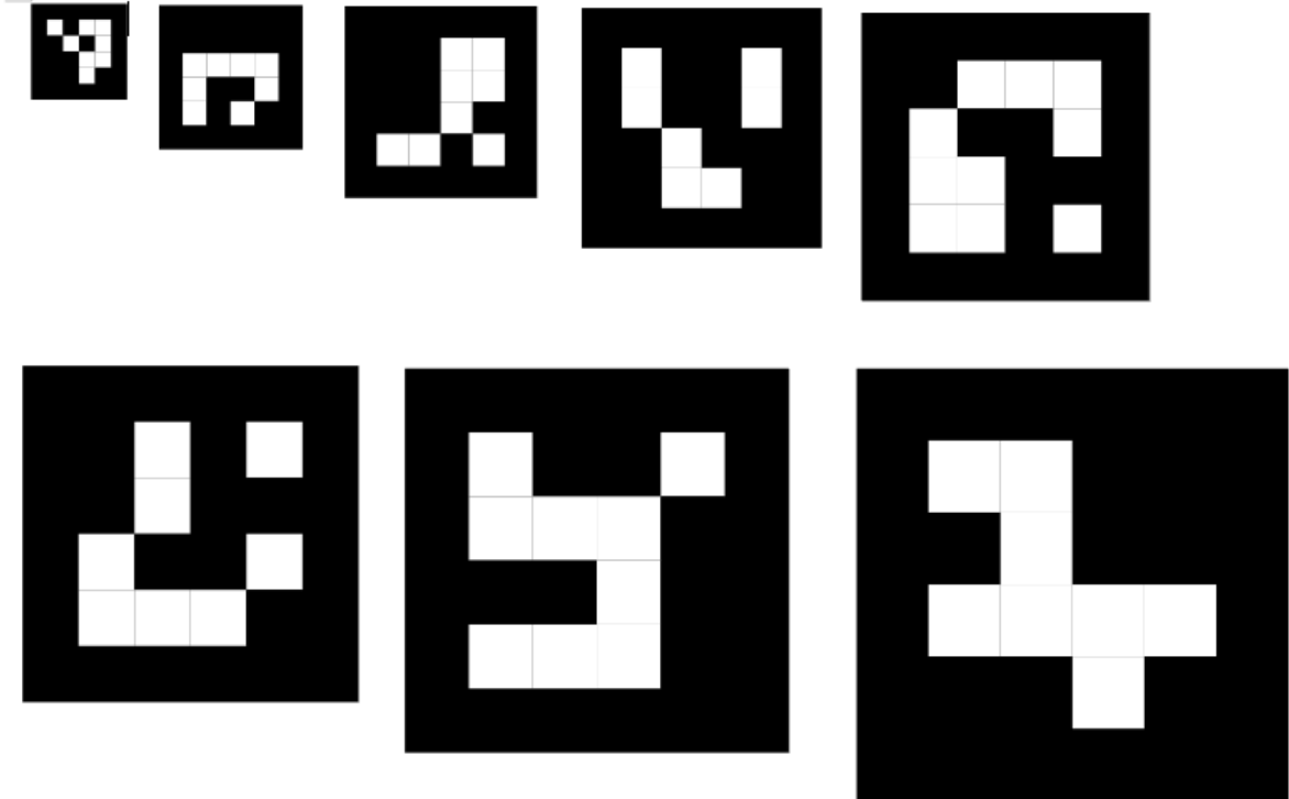
Figure H.2: Test sheet used for the testing of ArUco detection
