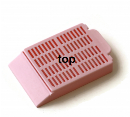
Figure 11: The sample is placed in the pink tissue cassette, with the part that was facing upward during compression testing, facing upward in the cassette (as indicated).
