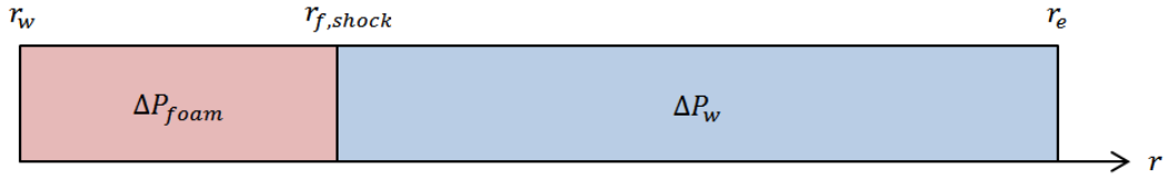
Figure 7: Gas Injection into a Single Layer Surfactant-Saturated Reservoir
