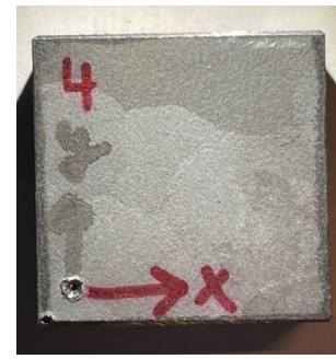
Fig. 15 Image of Sample 4 of a visually smooth section of the pipe wall. The size of the sample is 20 \times 20 \text{ mm}^2
