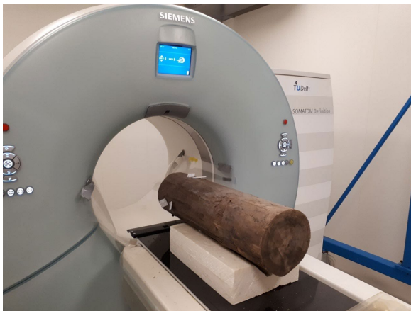
Figure 9: CT scanning test of retrieved timber pile
