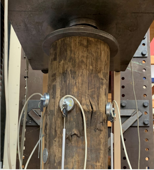
Figure 14: Failure in compression around knots
