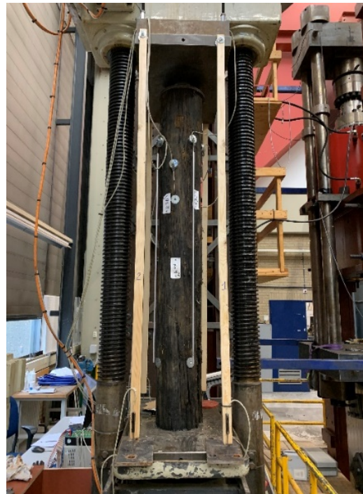
Figure 12: Large scale compression test set-up.
