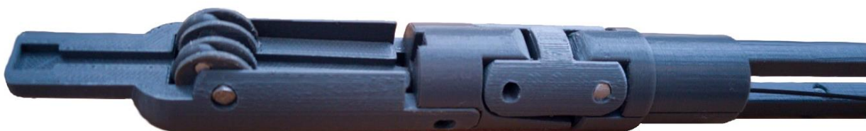
Figure 62: 3D printed prototype of the final design, 500% larger than the original.
