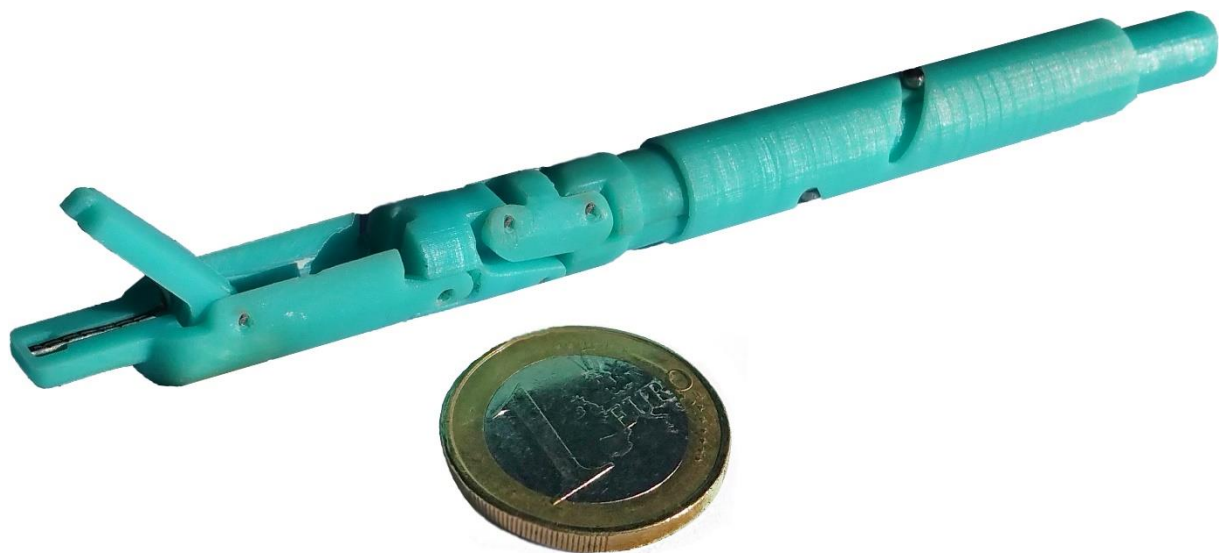
Figure 68: 3D printed prototype of the final design, 200% larger than the original.
