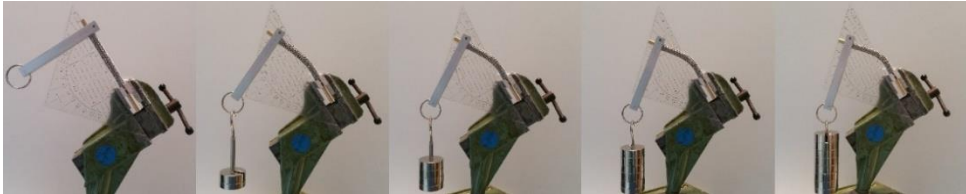
Figure 42: Amount of deflection under load.
