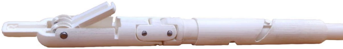
Figure 56: 3D printed prototype of final concept 500% larger than the original.
