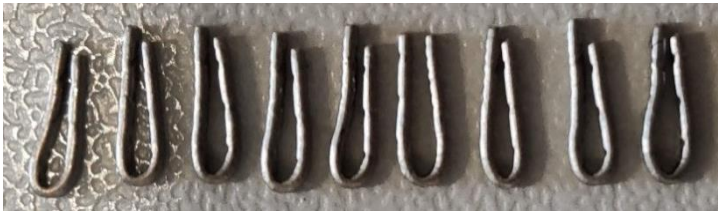
Figure 25: Results of the 9 bending trials.
