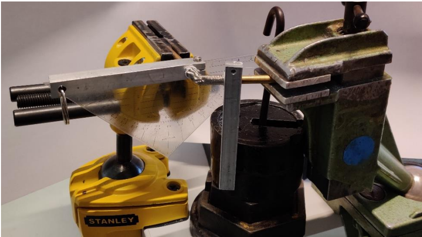
Figure 48: weakening of 4.5 mm woven steel tube.
