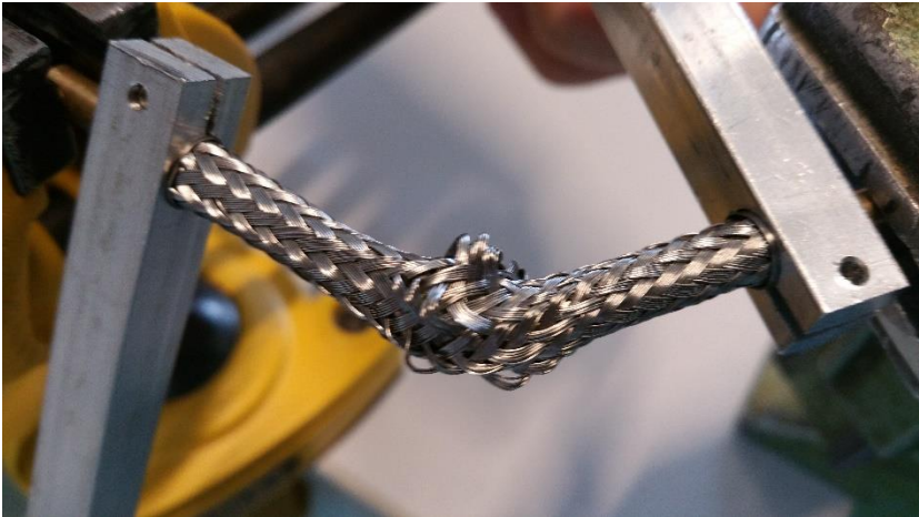
Figure 47: Failing of 10 mm woven steel tube.
