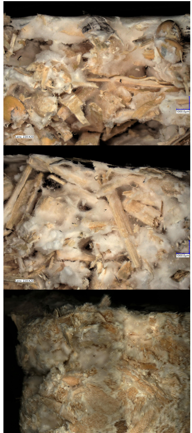
FIGURE 62 MICROSCOPIC IMAGES OF 3 SECTIONS: REGULAR HEMP/STRAW, HEMP/STRAW WITH EXTRA GROWTH PHASE, ECOVATIVE
