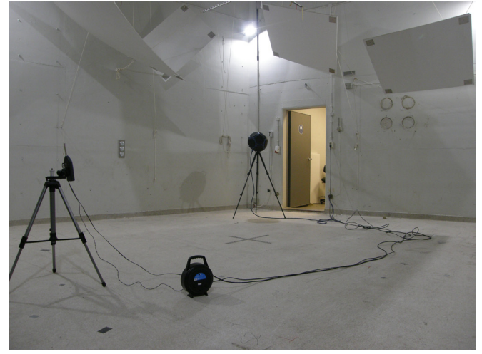
FIGURE 91 REVERBERATION CHAMBER, WITH DIFFUSERS, MICROPHONE AND OMNIDIRECTIONAL LOUDSPEAKER, AT THE FACULTY OF APPLIED SCIENCES, TU DELFT
