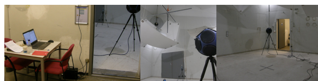
FIGURE 910 MEASUREMENT SETUP: LAPTOP CONNECTED THROUGH A HOLE IN THE WALL TO A MICROPHONE AND A LOUDSPEAKER
