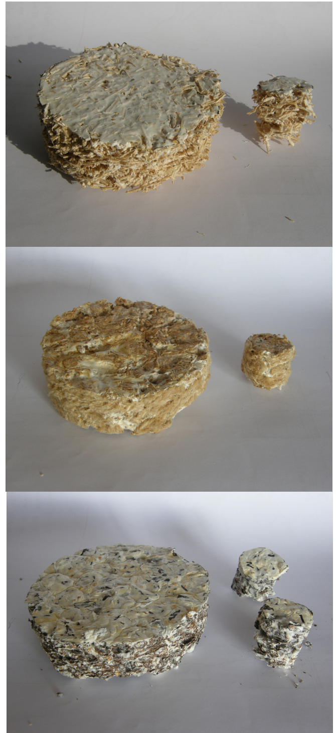
FIGURE 52 SAMPLES WITH HEMP/STRAW, CATTAIL AND CACAO SUBSTRATES
