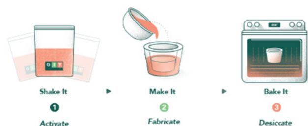
FIGURE 25: SCHEMATIC OVERVIEW OF THE GROWTH PROCESS BY ECOVATIVE
