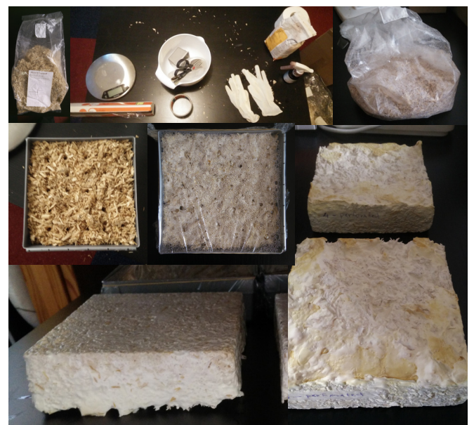
FIGURE 26 USE OF THE GROW-IT-YOURSELF KIT: SET-UP; BAG; GROWTH IN BAG; GROWTH IN SHAPE; DRYING; FINAL PRODUCT
