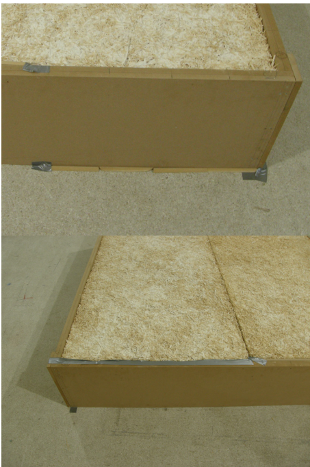
FIGURE 914 GAPS BETWEEN THE MOUNTING AND THE FLOOR OR THE PANELS ARE FILLED WITH MDF OR COVERED WITH DUCT TAPE
