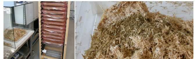
FIGURE 93 FILLING THE GROWTH SHAPES AFTER PASTEURISATION WITH ALREADY VISIBLE COLOUR DIFFERENCES
