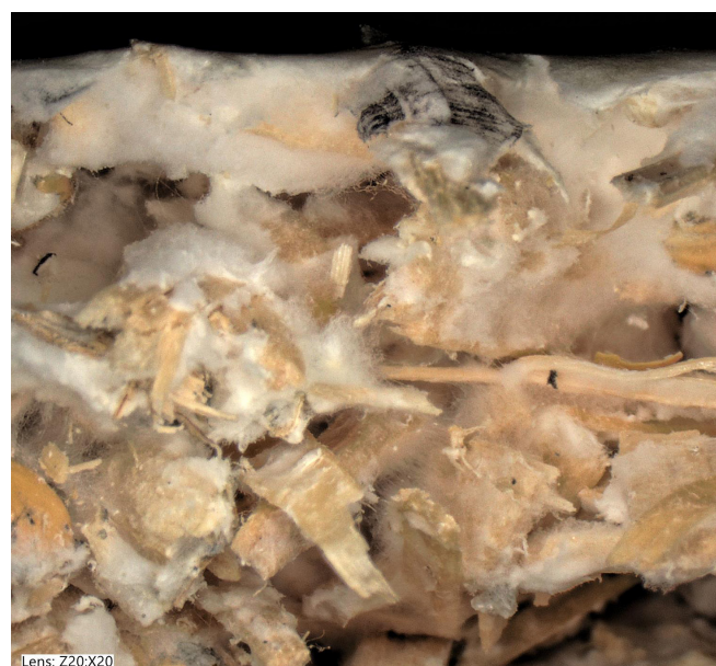
FIGURE 414 MICROSCOPIC IMAGE OF A HEMP/STRAW SAMPLE CROSS-SECTION
