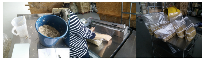
FIGURE 92 MIXING STRAW AND HEMP AND PUTTING THEM IN SEALED BAGS
