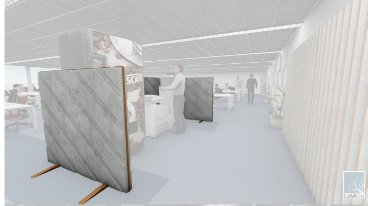
FIGURE 85 THE REGULAR PANEL: SINGLE PANEL AND PANELS WITH DISTANCERS FOR BROAD-BAND ABSORPTION
