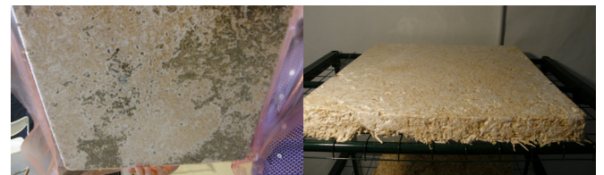
FIGURE 94 40 x 40 CM 2 PANELS WITH AND WITHOUT CONTAMINATION
