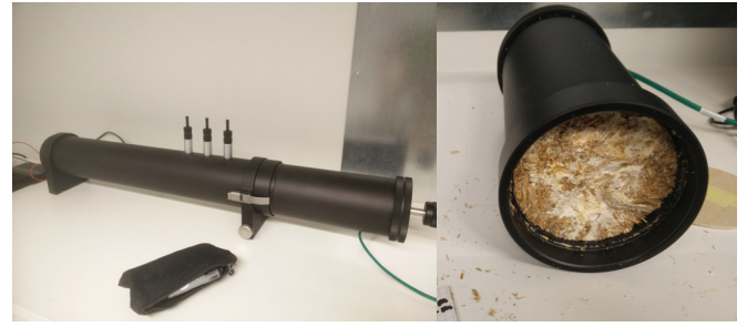
FIGURE 59 LARGE IMPEDANCE TUBE OF 100 MM DIAMETER
