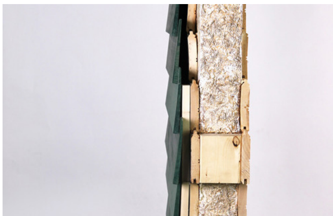
FIGURE 714 WALL MOCK-UP WITH MYCELIUM INSULATION BY ECOVATIVE
