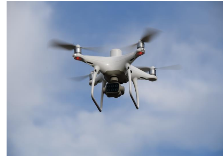
Figure 15. Acquisition in the field – Zenmuse L1 LiDAR & P4 Multispectral
