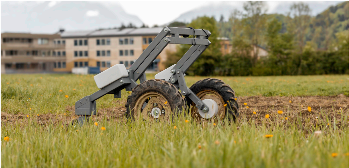
Figure 97: Cropkit IQ – Four-Lever Mechanism in Raised Position
