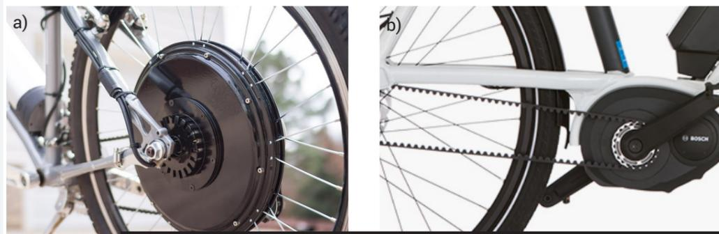
Figure 19. Electric bicycle systems. a) Hub motor, b) mid-drive motor.
