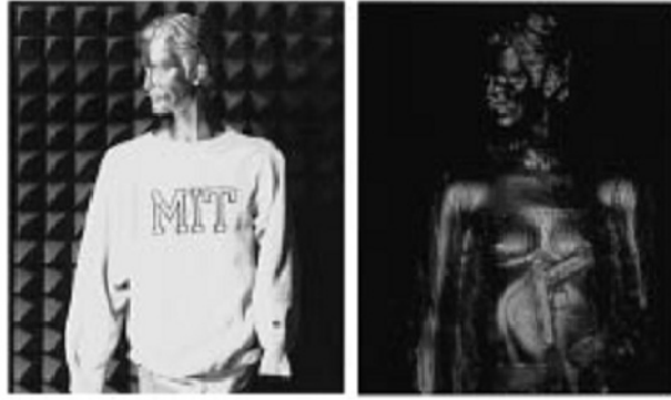
Figure 1.3.: Optical (left) and 110-112 Ghz image (MM wave on the right) of a clothed mannequin with a concealed Glock-17 handgun. Image from [13].
