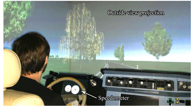
Fig. 7. The fixed-base driving simulator at the Faculty of Aerospace Engineering of the Delft University of Technology
