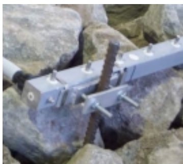
Figure 5.63: Clamps to fix the run-up gauges to steel bars driven into the outer layers of the breakwater.
