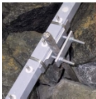
Figure 5.63: Clamps to fix the run-up gauges to steel bars driven into the outer layers of the breakwater.
