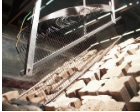
Figure 5.1: The novel digital step gauge installed in the flume of Flanders Hydraulics.
