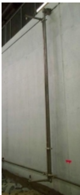
Figure 5.60: Capacitance type wave gauge.
