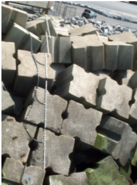
Figure 4.14: The five part run-up gauge mounted along the slope of the breakwater on top of the armour units.
