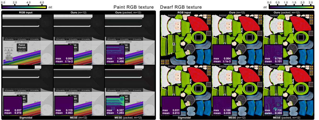
Fig. 11. Unconstrained texture uplifting. We uplift RGB textures and render under D_{65} . We show output for our method ( m = 12 coefficients), a low-bit packed variant, the sigmoidal [Jakob and Hanika 2019] and bounded MESE [Peters et al. 2019]. Mean and maximum \Delta E_{00} are listed for all outputs.
