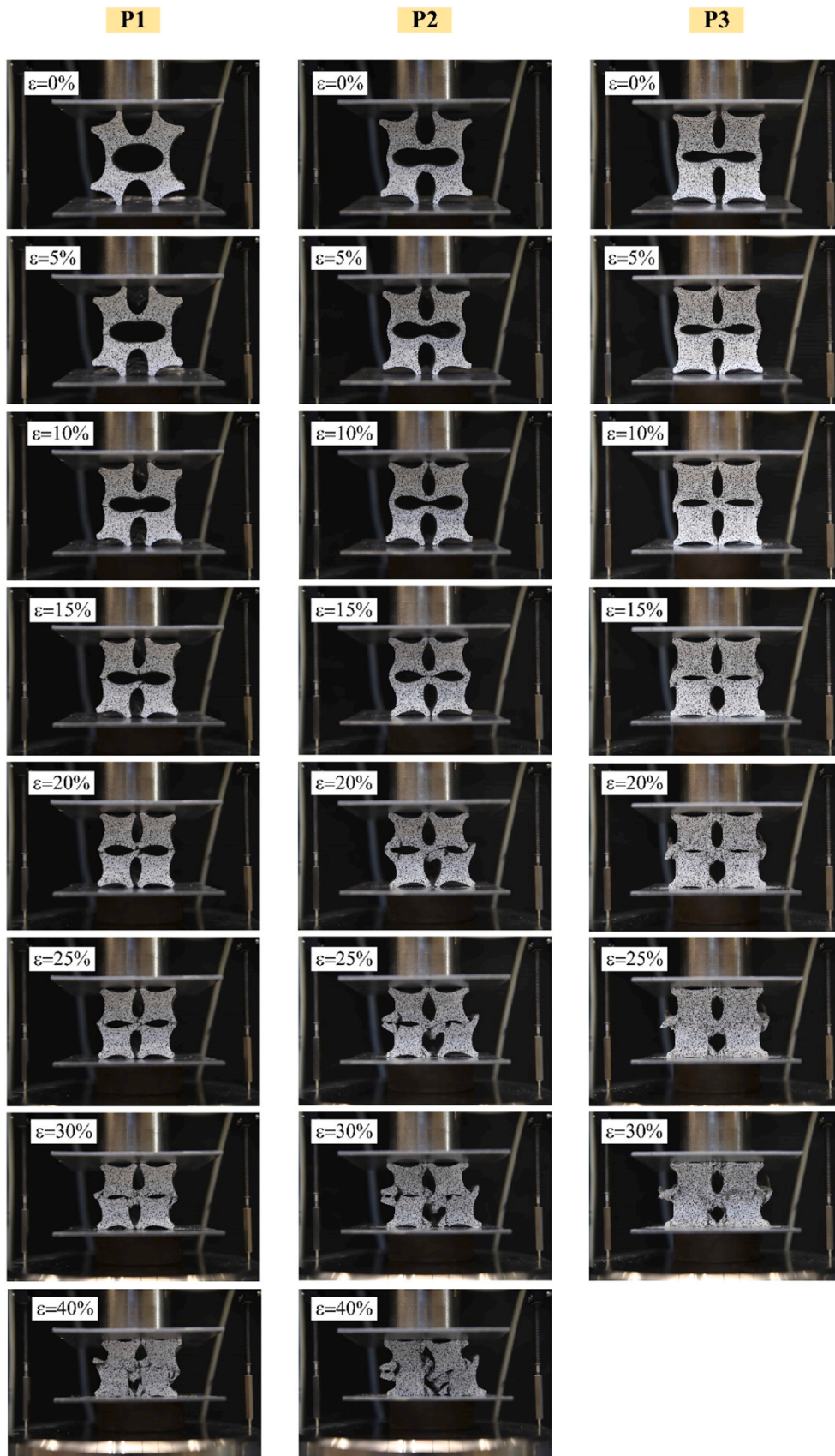
Fig. 11. The deformation process of ACCCs under compression.
