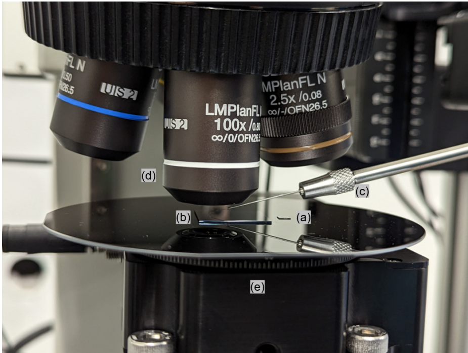
Figure 4.1: A photo of the pick and place setup. (a) is the diamond donor chip containing the diamond chiplets. (b) is the SiN receptor chip. (c) is the tungsten needle with a tip diameter of 200 nm. (d) is 100X objective with 400 nm resolution. (e) is the piezo stage with 47.6 nm step size.
